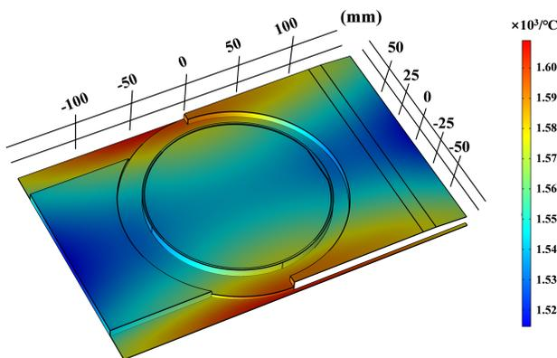
Fig. 3 Temperature distribution of reactor at steady-state equilibrium.
