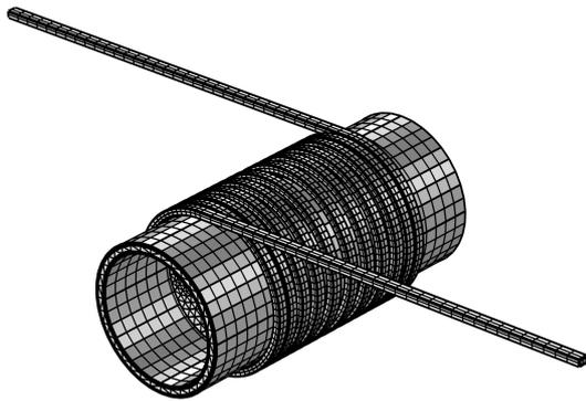
Fig. 2 FEM mesh of 3D model reactor.
