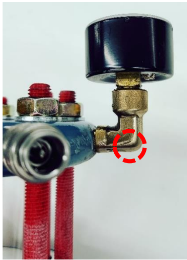
Figure A.17 Improvement of the cell with a smoothened L-shaped connection to the pressure meter. Red dotted circle is where BD occurred.
