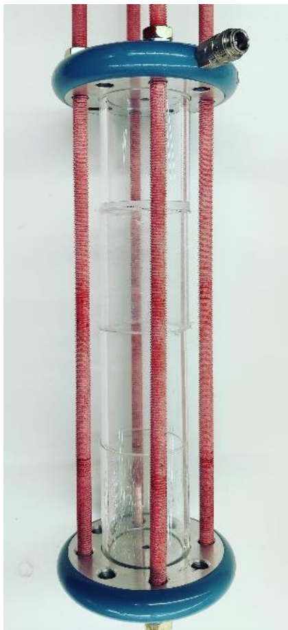
Figure A.19 Test cell with stacked cylinders, this test cell contains 4 cylinders.
