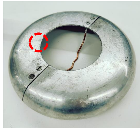
Figure A.18 Corona disk used for electrode grading. Red dotted circle is where BD occurred.
