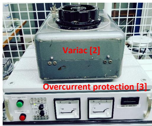
Figure 4.20 The variac and safety box used in the circuit to examine the PD characteristics of corona in C4-FN/CO 2 (5%/95%).
