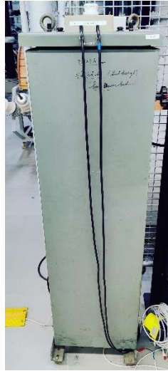
Figure 4.11 Variac used to regulate the applied voltage in the BD experiments.
