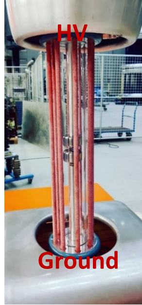
Figure 4.8 Added corona shields to mitigate corona discharges caused by the sharp contour of the DIL0 connections.
