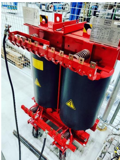
Figure 4.13 Inductor used to create resonance with the capacitive test cell.
