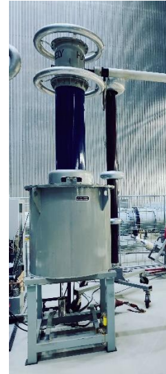
Figure 4.12 the step up transformer to step up the low regulated voltage to high voltage.
