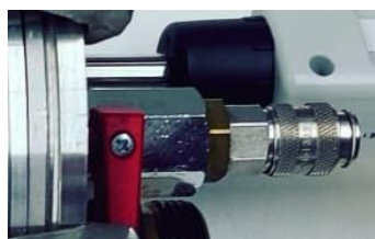
Figure A.25 A zoom-in of the red switch controlling the inlet flow of the gas on the mixing vessel.
