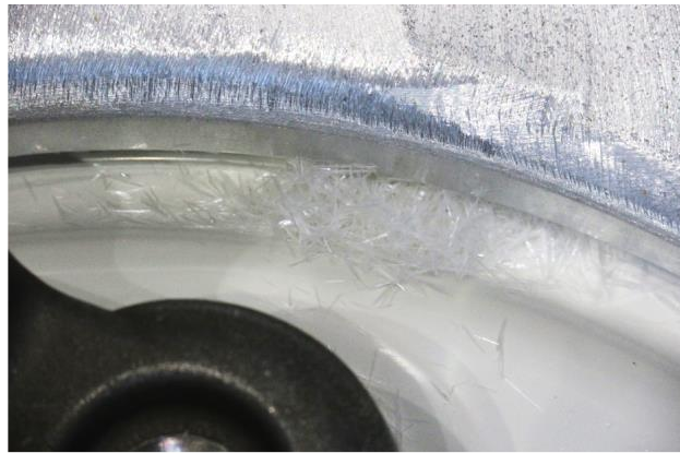
Figure 3.12 Crystals found in the VT after 800 days at 1,25x Un [3].
