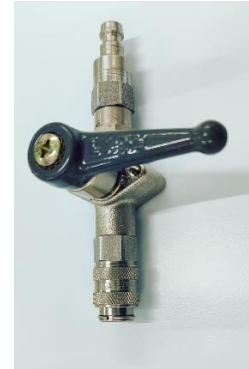
Figure A.29 Added grey switch to prevent problems occurring at step 7.
