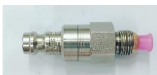
Figure A.26 The connection piece which enables the syringe to inject the water into the mixing vessel.
