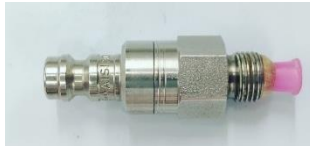
Figure 4.6 The connection piece which enables the syringe to inject the water into the mixing vessel.
