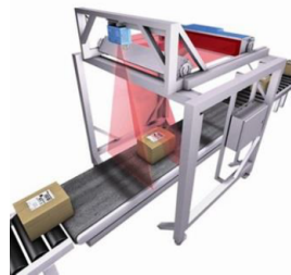
Figure 6.6: Automated (volume)scanning & weighing of box-size components
