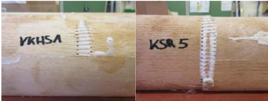
Figure 11: Half-pole finger joint HFJ (left) and complete cross-sectional finger joint (right)
