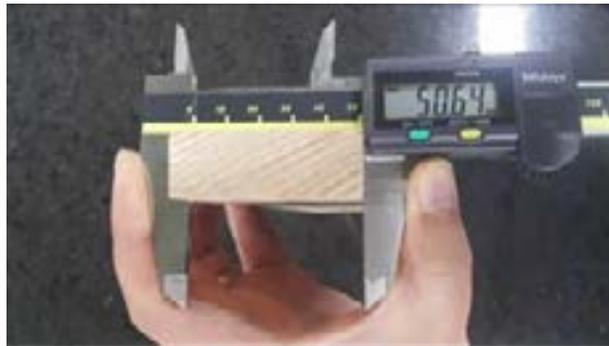
Figure 2: digital caliper (CD-20APX, Mitutoyo)
