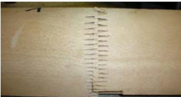
Figure 10: Half section with milled finger cuts
