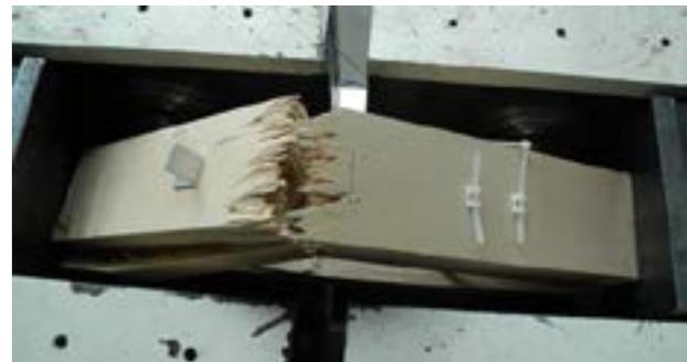
Figure 4: Compressive test apparatus and facies of failure on beech GLT.
