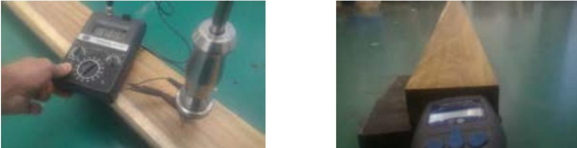
Figure 2: Measurement of moisture content and dynamic modulus of elasticity test.
