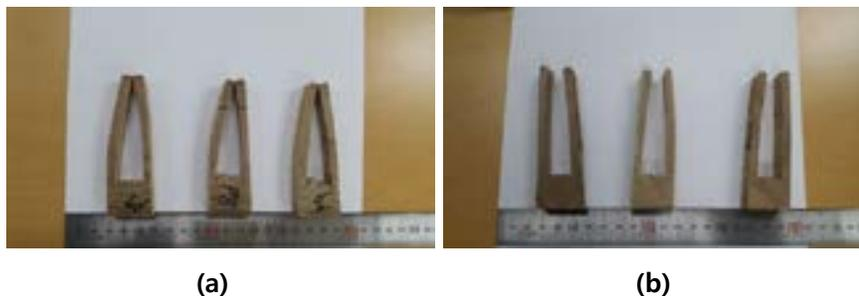
Figure 5: Drying stresses measured by prong test of KD board by prong test((a): 72hr, (b): after conditioning)
