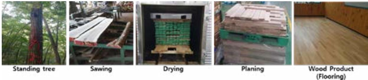
Figure 6: The production processing for oak flooring.
