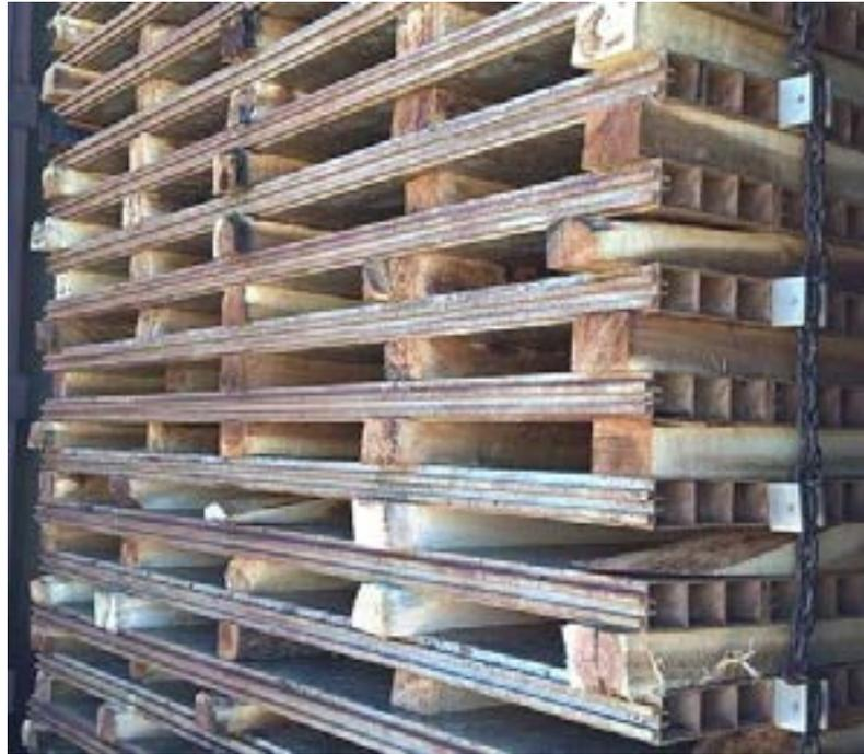
Fig. 1. A set of acacia boards (60×80×1200 mm) after the compression and thermal modification process.
