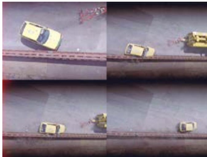
Figure 8. Top view with a high speed camera of the car impact on the guardrail, Full-scale test with a 900 kg car (Test TB 11 according to EN 1317)
