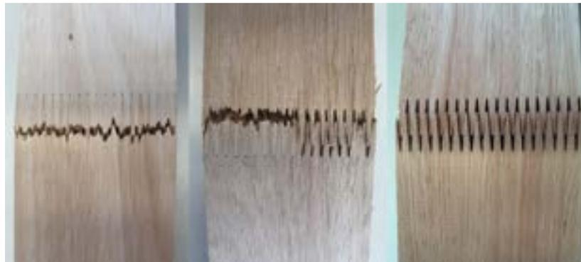
Figure 2: Failure modes of finger-joint lamellas: Mode 1 (left), Mode 2 (center) and Mode 3 (right)
