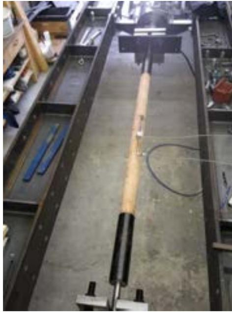
Figure 9: Test setup of a full-sized CLHS
