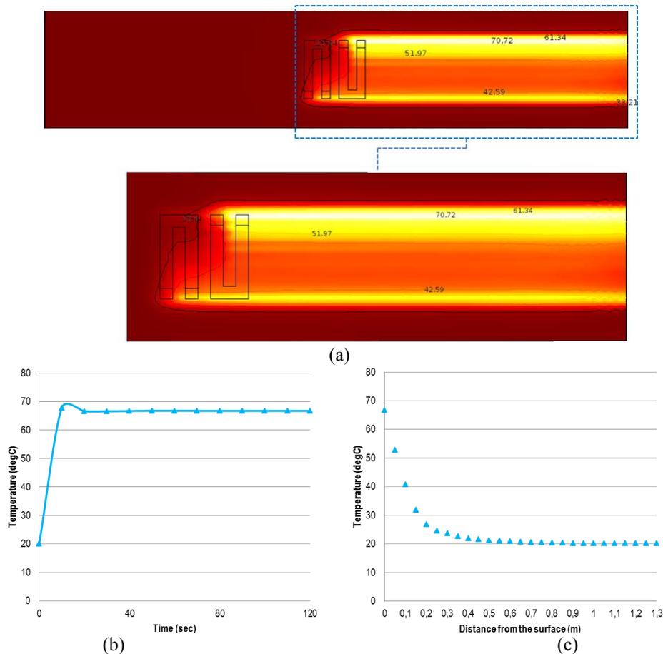
**FIGURE 6 FEM results of induction heating on pavement: (a) thermal field distribution at pavement surface, (b) surface temperature development of pavement and (c) temperature distribution in pavement after 120 seconds of induction**
