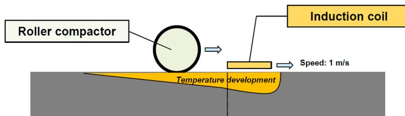
**FIGURE 1 IH-compaction process**
