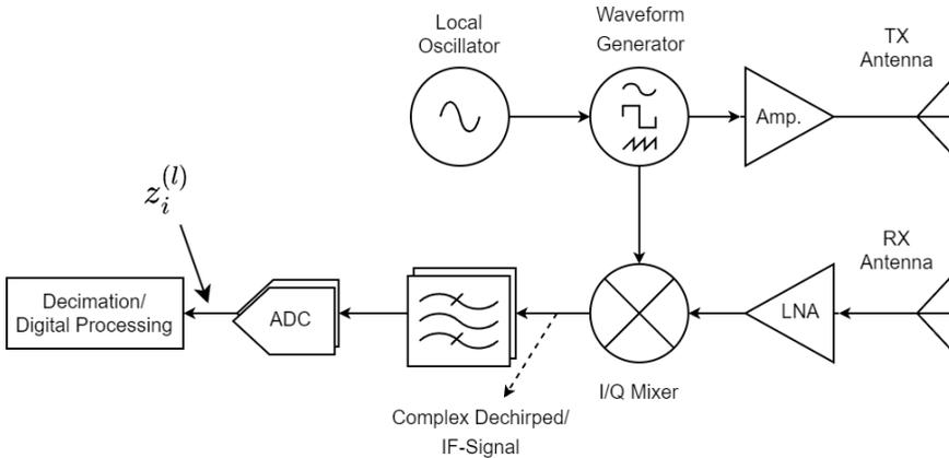
Figure 2.4: Simplified example block diagram of a FMCW transmit and receive frontend. Based on [81], [82]
