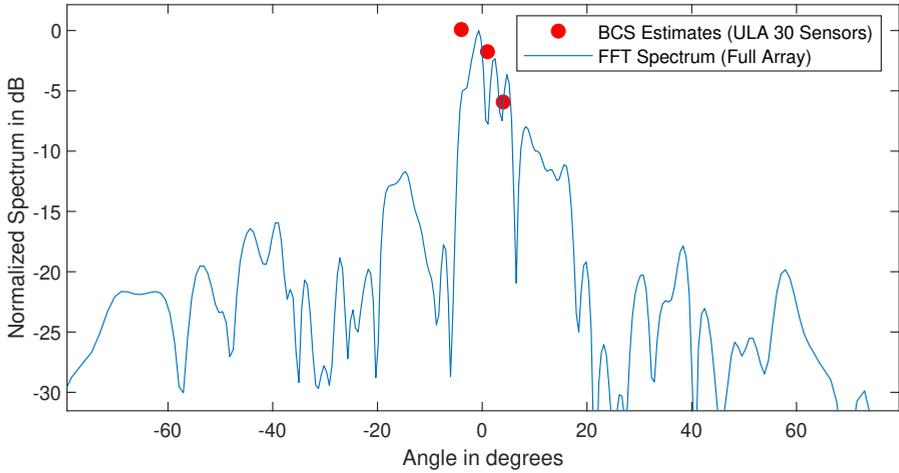
(a) BCS estimates using a physical ULA based sparse array with 37 sensors.
