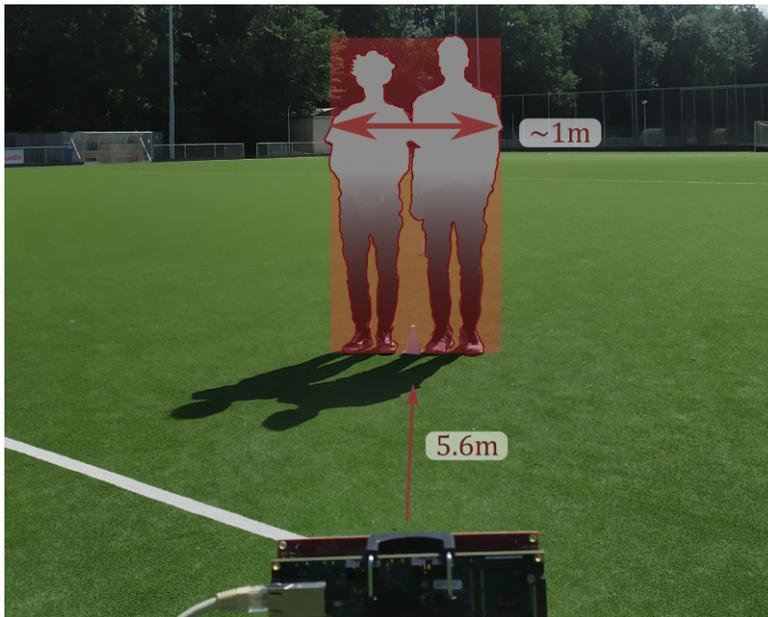
Figure 4.12: Measured scene of 2 persons standing closely together to form an extended target. The span from shoulder to shoulder is about 1 meter, corresponding to around  $10^\circ$  angular spread.
