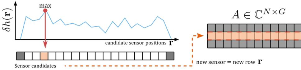
Figure 2.9: Visualisation of the concept of checking each candidate sensor location and adding the one which achieves  $\max \delta h$ .
