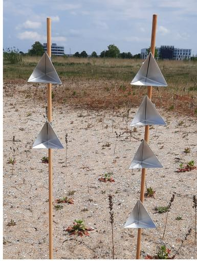
Figure 4.7: Composition of corner reflectors to achieve different target RCS values.
