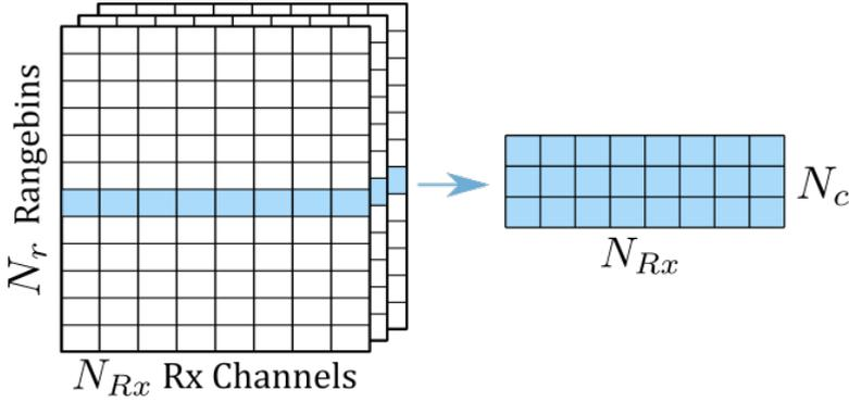
Figure 2.3: Radar Datacube on the left and the extracted range bin information (in blue). The different layers of the data cube indicate the data captured from  $N_c$  consecutive chirps (in slow time). The x-Axis shows the data for the different receiver channels, which are denoted here as  $N_{Rx}$  and can be either formed by a physical or a virtual array.
