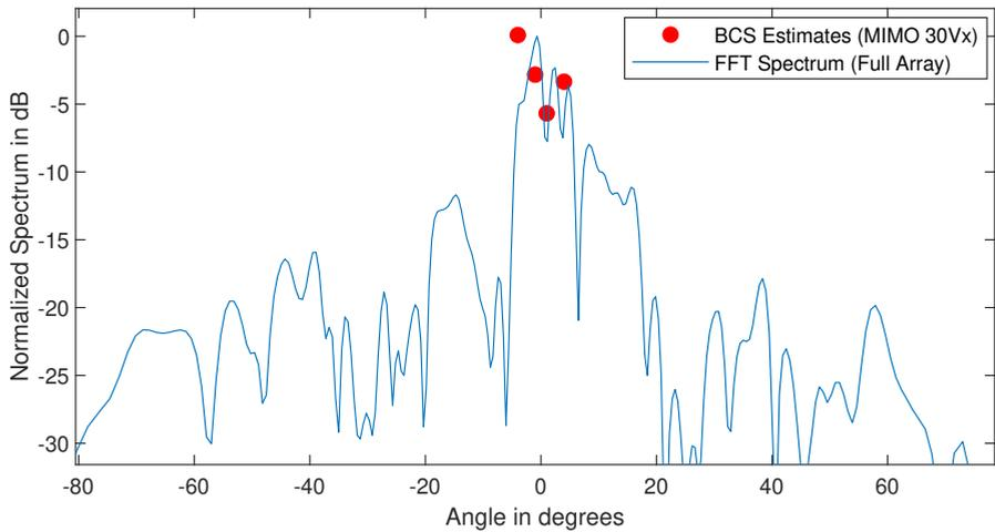
(b) BCS estimates using a MIMO based sparse array with 6 physical transmitters, 5 physical receivers and resulting 30 virtual receivers.
