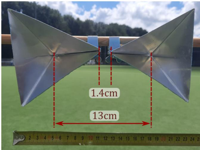
(b) Close-up photo of the two corner reflectors at their closest spacing of 13 cm (measured from their centres), corresponding to  $1.33^\circ$  angular separation.
