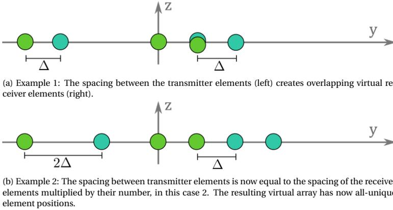
Figure 2.6: Two examples showing the concept of the MIMO array. It visualises the design choices regarding the placement of the sensors.
