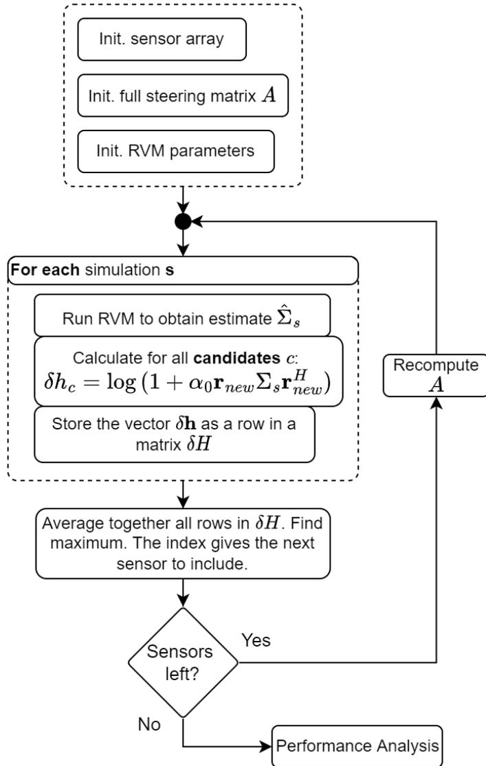
Figure 3.1: Overview block diagram of the entropy based sensor inclusion algorithm for the ULA case. It is important to note, that the algorithm will run until all possible sensor positions are included. A stopping criterion (i.e. maximum number of antennas) could be added depending on the use case.
