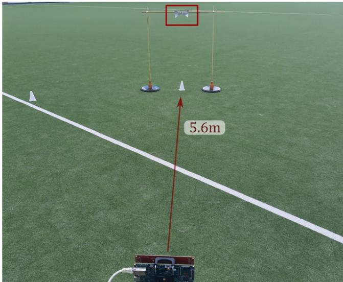
(a) Setup of the second capture, showing the radar in the front and the corner reflectors in the back.
