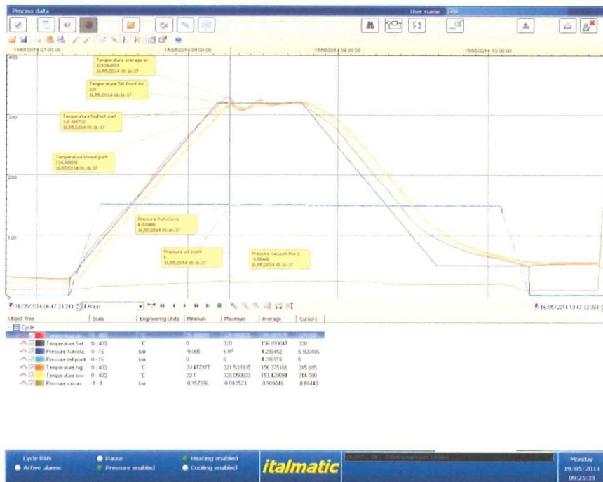
Figure C-2: Autoclave cycle in which the PEKK ED is consolidated.
