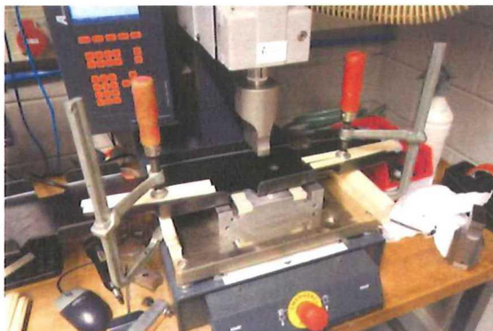
Figure 5-16: Clamping of the rib onto the anvil of the Rinco 3000. The rib is simply clamped with two glue clamps. Wooden sticks are placed in between to prevent damage.
