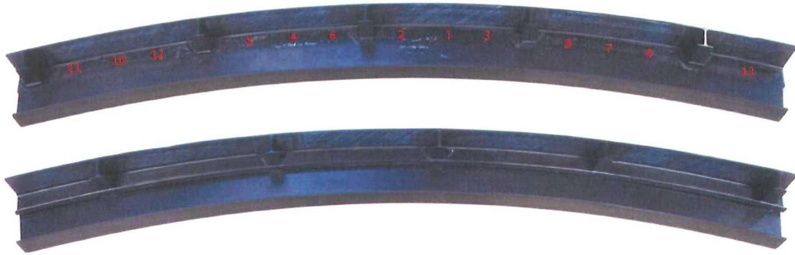
Figure 8-3: The fuselage frame welded to a section of the orthogrid panel. Upper: top-view of the fuselage frame; lower: bottom-view of the fuselage frame. The red numbers indicate the locations and sequence of the spot welds. See Figure G-1 for a larger version of this picture.
