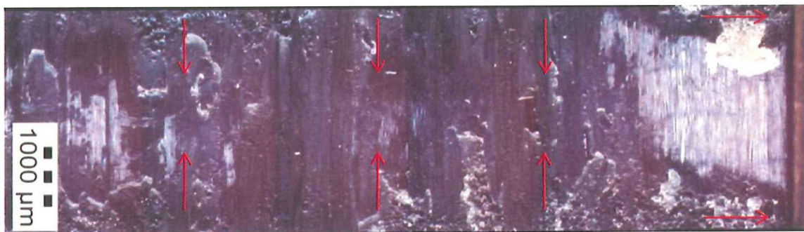
Figure 4-9: Merged flow fronts in a sample clip welded at 800 [J]. Flow directions are indicated with the red arrows.
