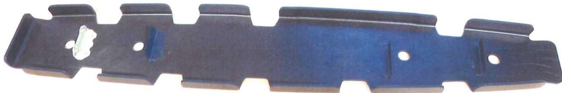
Figure 5-18: CFRTPC clips ultrasonically welded to a CFRTPC rib. The left-most clip is the original aluminum clip and it is riveted to the rib. The second clip is a CF/ PPS clip and the two right-most clips are CF/ PEKK clips. The CF/ PPS clip is welded with PEKK EDs.
