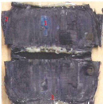
Figure 7-7: The related fracture surfaces of USW140805-06 clamped at 3.5 [cm] and with a torque of 2.5 [Nm]. There are 1) resin rich areas; 2) fiber squeeze-out near the side edges; and 3) voids on one side of the weld.
