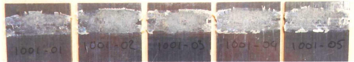
Figure 4-39: Fracture surfaces of five validation samples welded in the same conditions with 720 [J]. The fracture surfaces are similar in terms of area and failure mode as expected.
