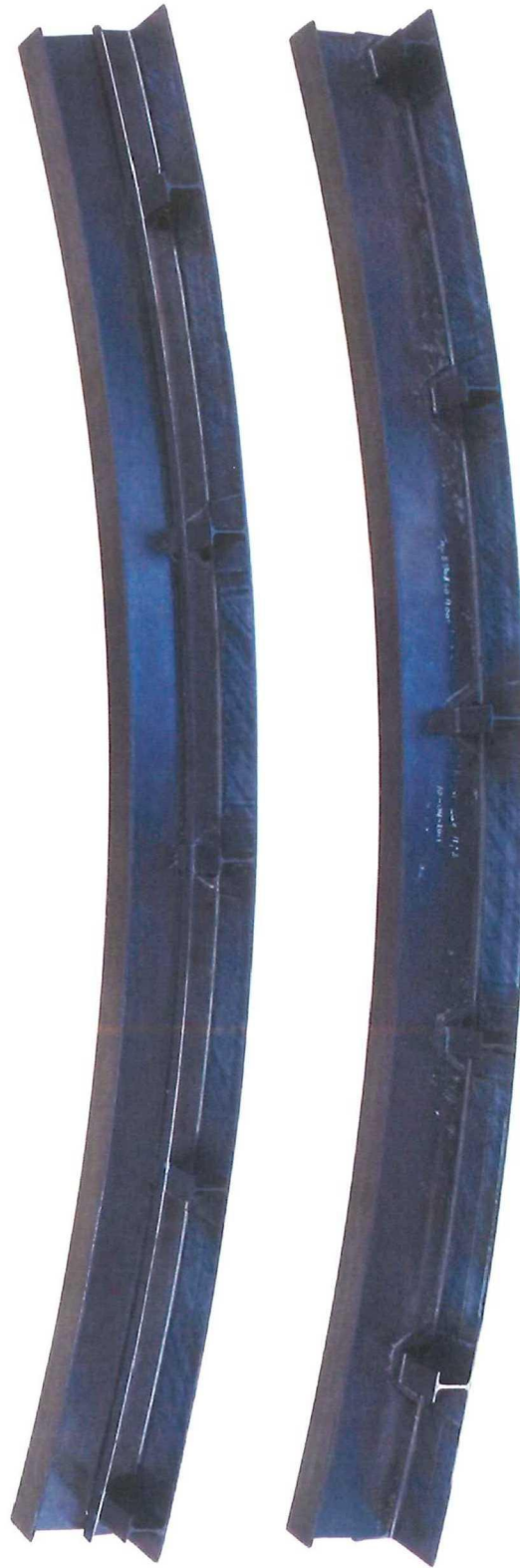
Figure G-1: A fuselage frame ultrasonically welded to a section of the orthogrid panel. Left: bottom view; right: top view.
