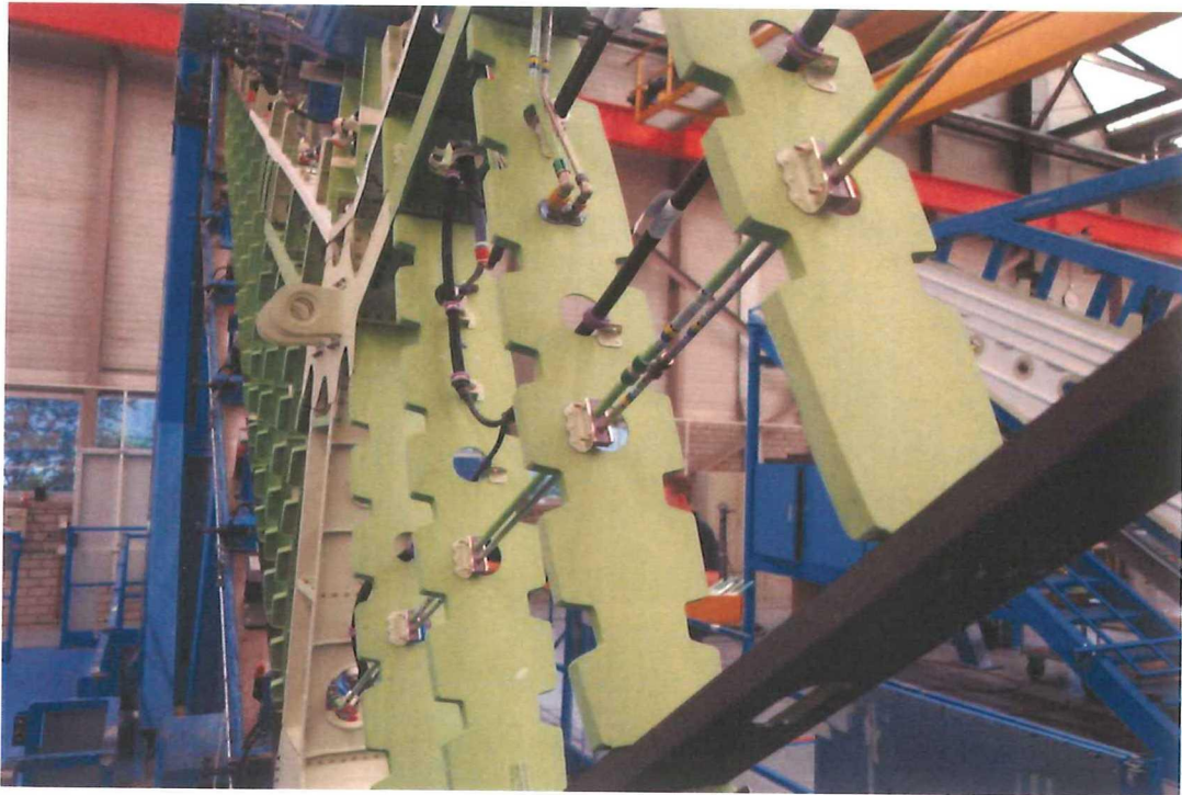
Figure F-1: Horizontal stabilizer of the Gulfstream G650 being assembled at Fokker Aerostructures in Papendrecht. Various clips are riveted on the ribs.
