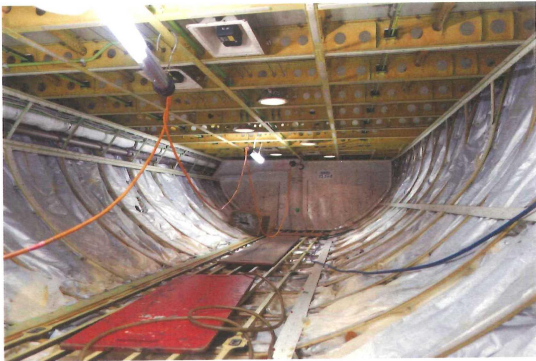
Figure F-3: Cargo hold of Boeing 737-800 being maintained by KLM Engineering & Maintenance. Numerous system clips can be seen that could possibly be welded in case the load carrying beams of the cargo floor were made of CFRTPCs.
