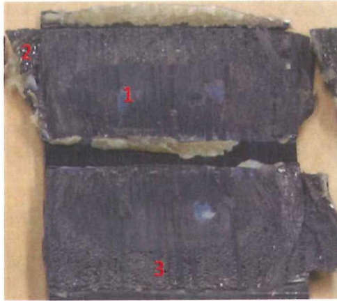
Figure 7-5: The related fracture surfaces of USW140827-05 clamped at 6 [cm] and with a torque of 2.5 [Nm]. There are 1) two resin rich areas in the middle; 2) fiber squeeze-out near the side edges; and 3) voids on one side of the weld.
