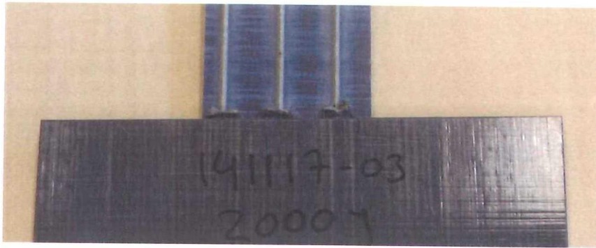
Figure 6-7: Sample clip USW141117-03 welded with 2,000 [J]. The triangular EDs are integrated in the upper sample. Squeeze out of ED and fibers is observed.
