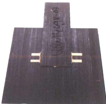
Figure 3-7: Sample clip welded with two ED strips at 2,000 [J].
