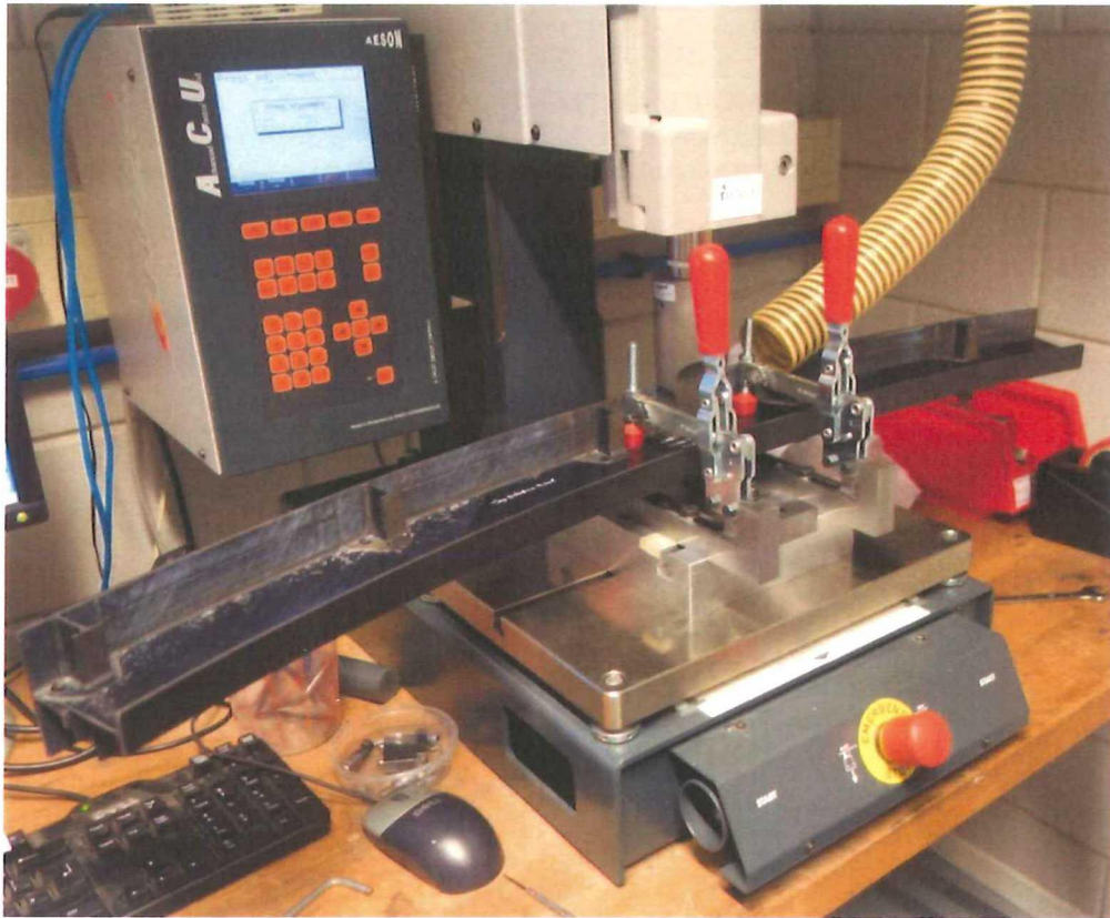
Figure G-4: The fuselage frame and the orthogrid panel clamped in the Z51430 fixture.
