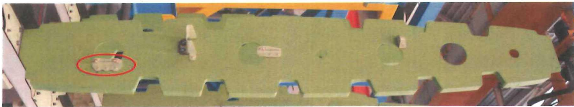
Figure 5-1: Original position of the aluminum clip on a rib of the horizontal stabilizer of the G650, as indicated by the red ellipse. The clip is fastened by three rivets.
