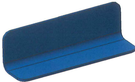
Figure 5-3: Composite clip based on the dimensions of the original aluminum clip. The clip is welded to the rib. The floating nuts could be integrated in the design or welded as well as there are already thermoplastic floating nuts.
