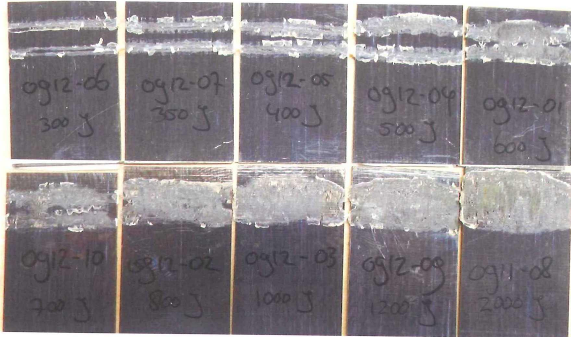
Figure 4-3: Fracture surfaces of sample clips in the order of the amount of energy used to weld. The two molten ED strips are merged between 700 [J] and 800 [J] and become one weld.
