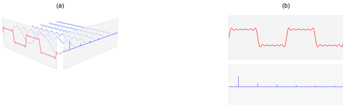
Figure 2.2: Time (red) and frequency domain (blue) representation of a waveform signal. (image adapted from [37])
