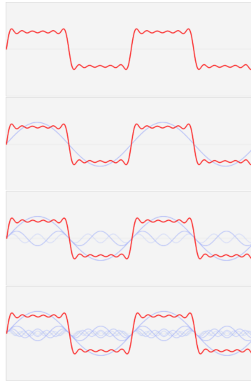
Figure 2.1: Sine and cosine decomposition of a waveform. Red represents the signal wave form. Blue represents the sines and cosines. (image adapted from [37])
