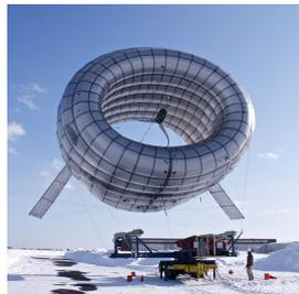
Figure 5.2: Airborne turbine [3]
