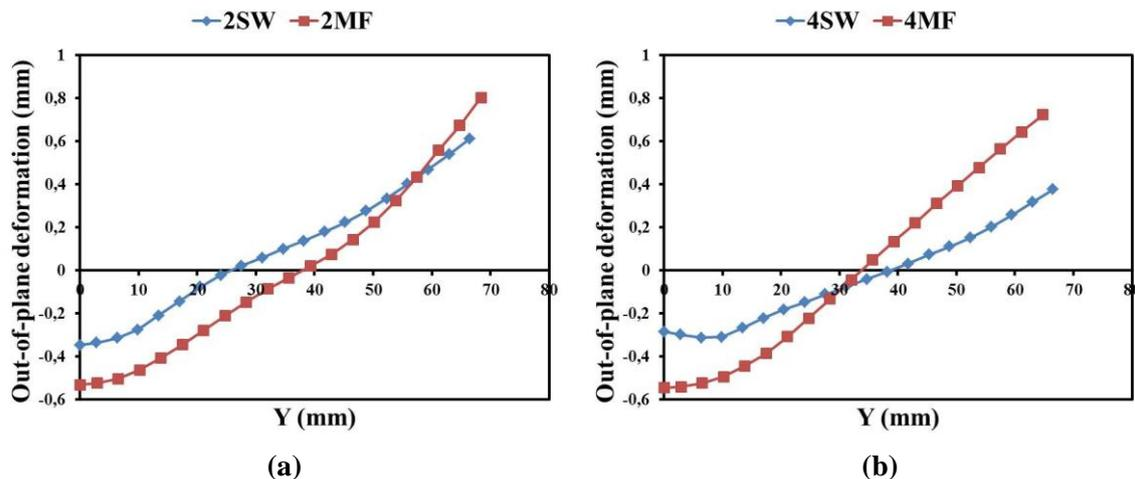
**Figure 9.** Comparison of out-of-plane deformation of the joint overlap under 7000N load between the MSW and the MMF joints with different number of spots/fasteners: (a) 2 spots/fasteners; (b) 4 spots/fasteners.
