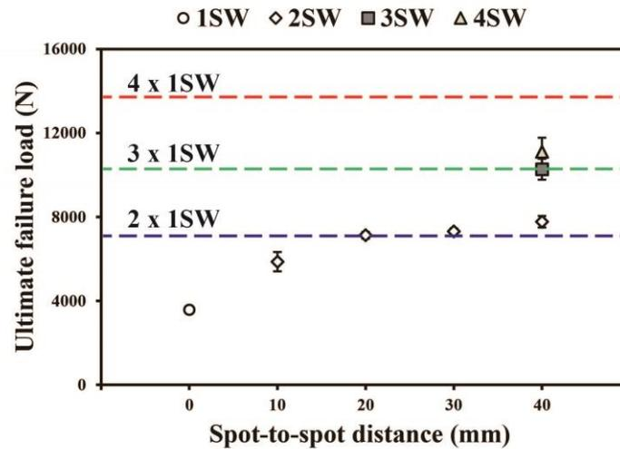
**Figure 7.** The increase of the UFL of MSW joints when increasing the spot spacing and the number of welded spots. Blue, green and red dashed lines indicate the two, three and four times of the UFL of 1SW joints, respectively.
