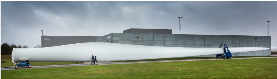
Figure 1.2: The 58.7 m GloBlade® 3 blade being transported with cradles in the factory yard at Lunderskov, Denmark. Source: LM Wind Power.
