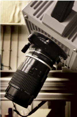
Figure 3.4: Scheimpflug adapter used in the PIV campaigns, located between the camera body and the lens.
