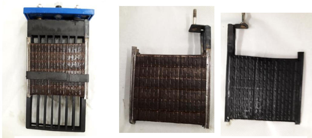
Figure 16. Battery out of container (a), nickel (b) and iron (c) electrode
