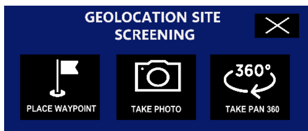
Figure 3.45: Prototype I: Geolocation Site Screening Menu with three options: placing a waypoint, taking a photo and taking a panoramic 360 photo.
