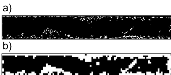
Figure 3.5: a) Segmented porosity cross-section on the xy plane, where pores are highlighted in white; b) same cross-section after max-filtering with a cubic element of 15 voxels side, corresponding to approximately 1.5 times the fibre diameter.
