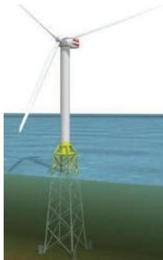
Figure 2.2 Hybrid Support Structure for Offshore Wind Turbine [5]
