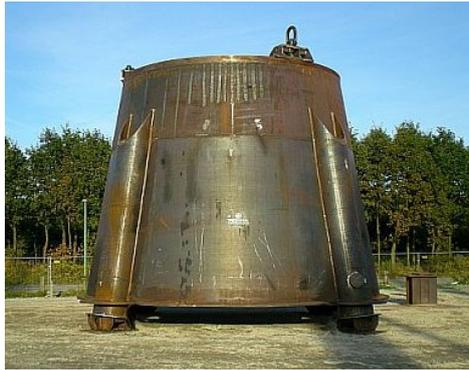
Figure 2.6 Transition Piece of REpower Jacket [8]
