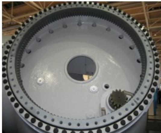
Figure 3.13 Bolting Connection of Yaw Bearing and Cylinder Flange [22]
