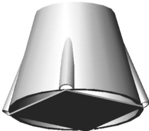
Figure 4.4 Cone-strut Transition Piece Model
