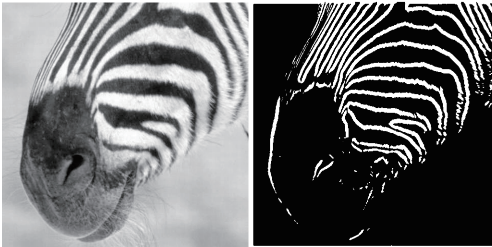
Figure 2.2: An example of image filtering. The left image is original image. The right image is generated after convolving edge detecting filter with original image.
