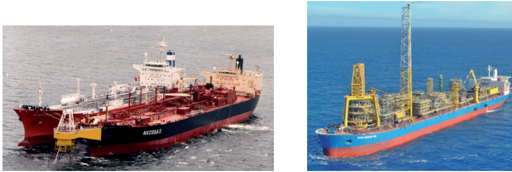
Figure 4.5: Left: SbS arrangement (FLNG with external turret); Right: FPSO - internal turret [33]
