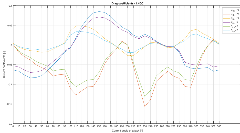
Figure 6.25: Drag coefficients for LNGC in fully loaded (FL) and ballast (B) condition
