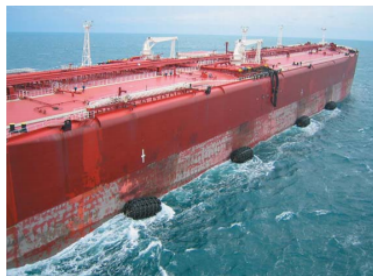
Figure 6.18: Pneumatic Fenders placed along the vessel [6]
