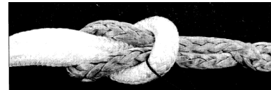
Figure 6.15: Tail-wire connection using 'cow hitch' method [30]
