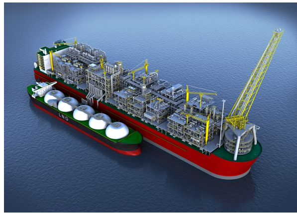
Figure 1.1: Side-by-side offloading operation[41]
