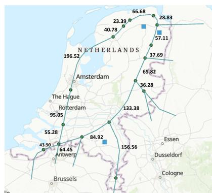
**Figure B.1:** Length of pipeline network between several nodal points in km
