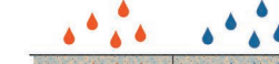
Fig. 3.5.1.7 Soil can gain / lose heat when it comes in contact with water of different temperature.
