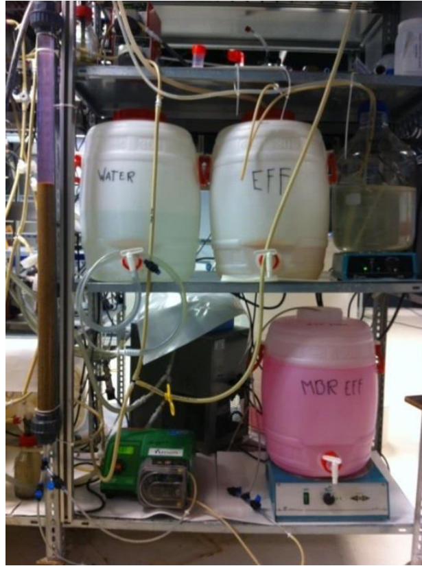
Figure 5.11 Ion Exchange set up, treating actual AnMBR effluent
