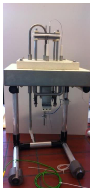
Figure 9.1 a. (left)The Open Flanges Set up in oven b. (right) the Open Flanges set up without oven
