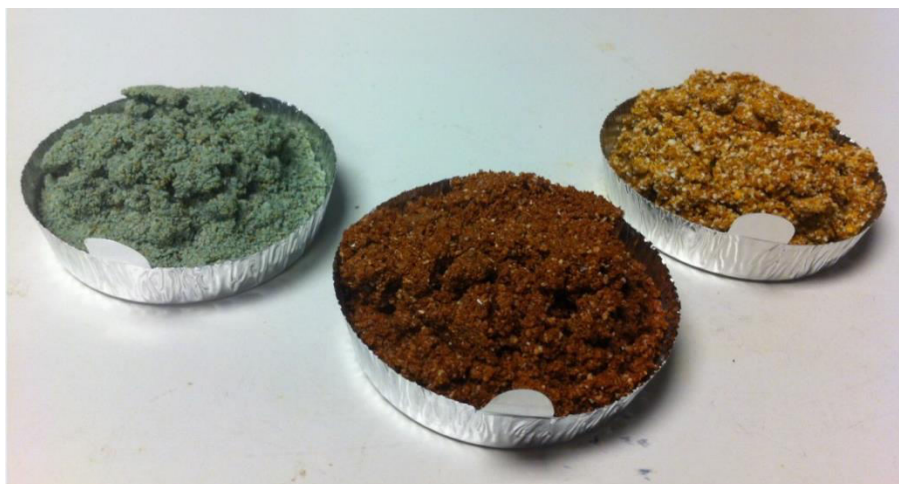
Figure 5.1 The three types of zeolites (Clinoptilolite (green), Clinoptilolite T (red) and Chabazite (yellow))
