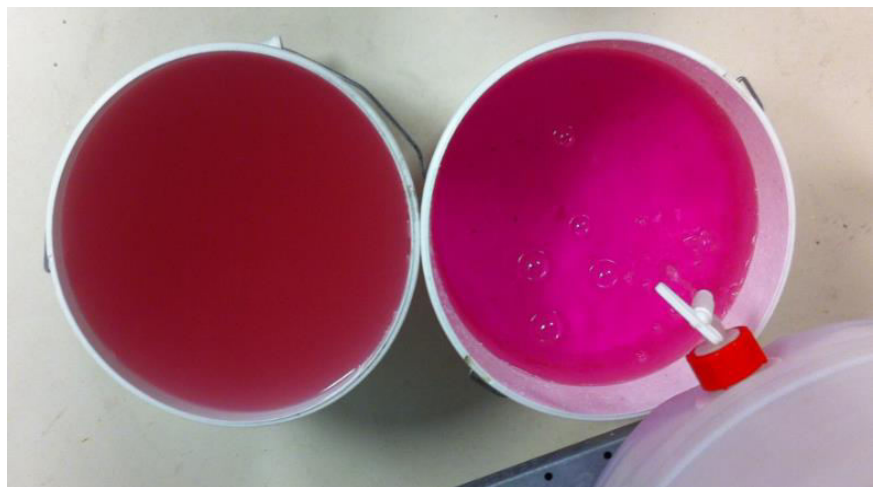
Figure 3.3a: reactor in operation, clearly showing particles moving up with the biogas and settling continuously. b (right): UASB effluent without membrane (left) and with membrane
