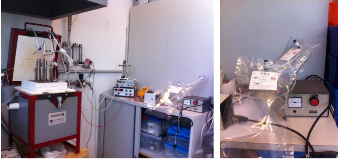
Figure 9.8 Set up used for tests with biogas as the fuel
