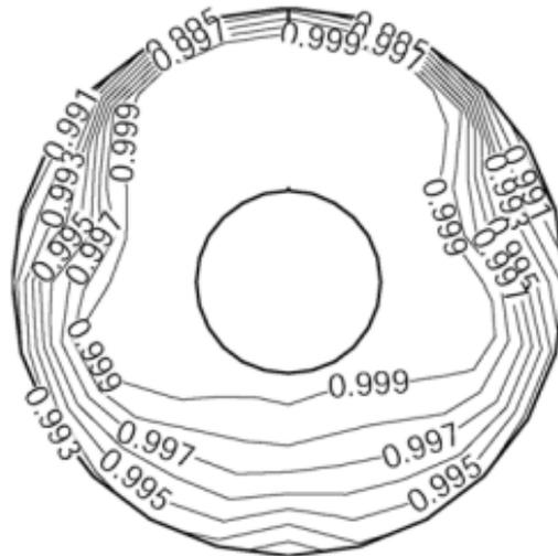
Figure 15: Total pressure ratio contour plot with AFC, DC60 = 4.6% [26]
