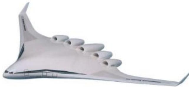
Figure 11: BWB using distributed propulsion with BLI [24]
