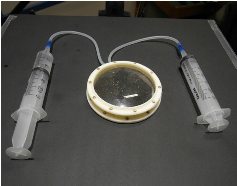
Figure 5 Aspects of the adaptive fluid lens and sunlight redirecting system prototype in 1:10 scale.
