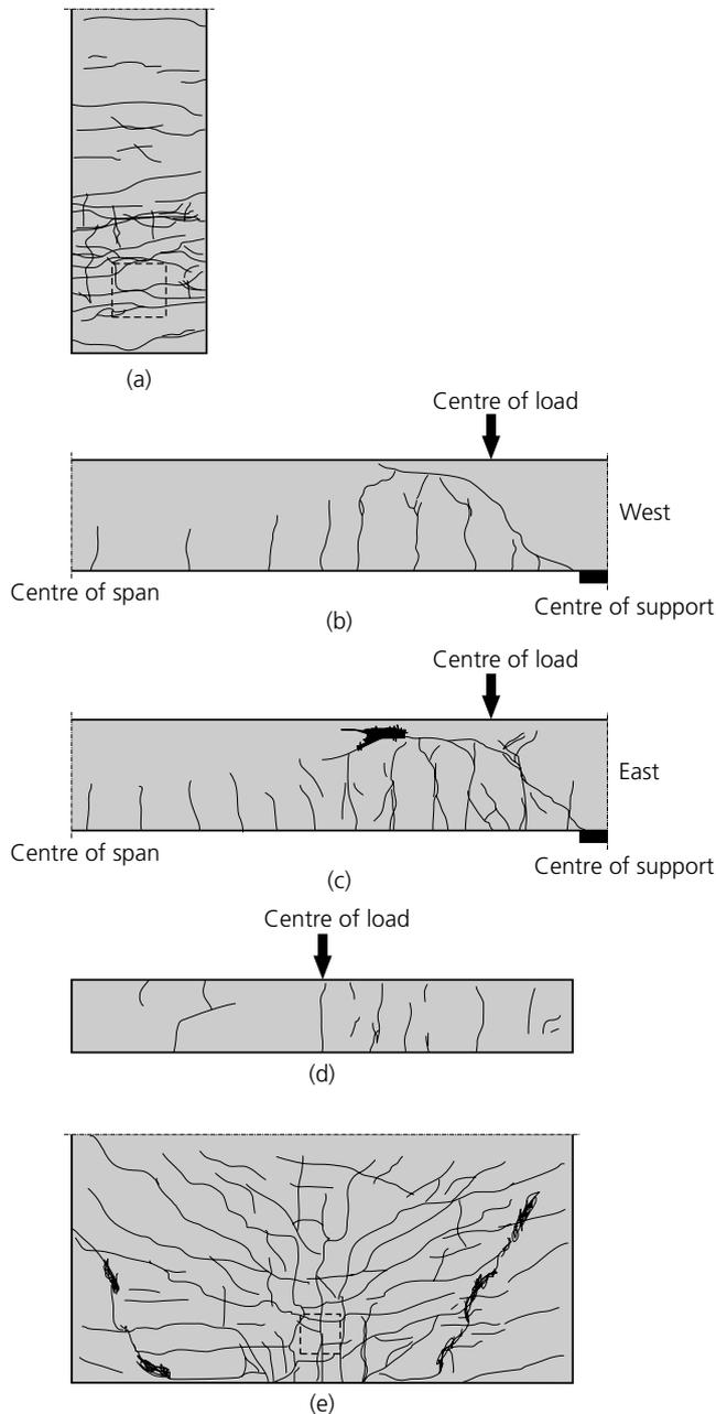
Figure 1. One-way shear: cracks after failure of BS2T1 (Lantsoght *et al.*, 2014): (a) bottom face; (b) west side face; (c) east side face. Two-way shear: cracks after failure of S9T1 (Lantsoght *et al.*, 2013c): (d) front face; (e) bottom face
