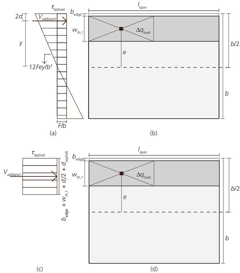
**Figure 8.** Model for contribution of increased loading in the first heavily loaded lane assuming a triangular stress distribution over the support: (a) assumed stress distribution  $\tau_{\Delta q_{load}}$  due to load and moment from eccentricity of load; (b) sketch of top view with
