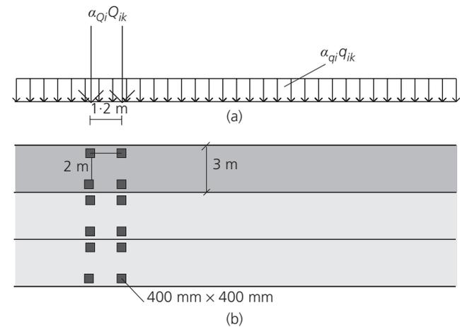
**Figure 3.** Traffic loads according to NEN-EN 1991-2:2003 (CEN, 2003): (a) side view; (b) top view
