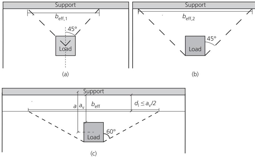
**Figure 2.** Effective width (a) assuming 45° horizontal load spreading from the centre of the load ( $b_{eff1}$ ) and (b) assuming 45° horizontal load spreading from the far corners of the load ( $b_{eff2}$ ); (c) top view of slab as prescribed by Model Code 2010 (fib, 2012)
