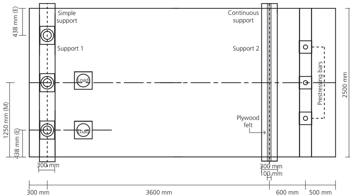
**Figure 5.** Top view of test setup for slabs under a concentrated load: supported by elastomeric bearings on the left and supported by a line support on the right. E indicates position of concentrated
