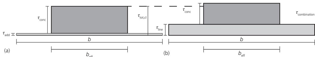
**Figure 6.** Superposition of shear stress due to a concentrated load over the effective width to the distributed load over the full slab width: (a) concentrated load only; (b) concentrated load and line load
