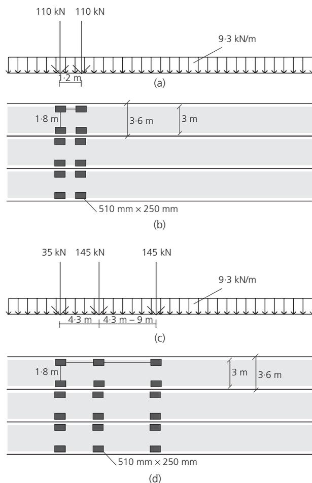
Figure 4. Loading as prescribed in Aashto (2015) with design tandem ((a) side view and (b) top view) and with design truck ((c) side view and (d) top view)
