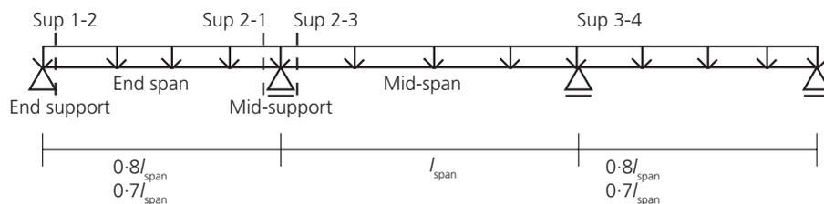
Figure 9. Considered sections for a typical three-span bridge
