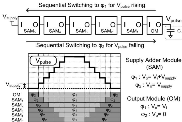
Figure 2.17: The 7-level supply multiplying pulser and operational concept.
