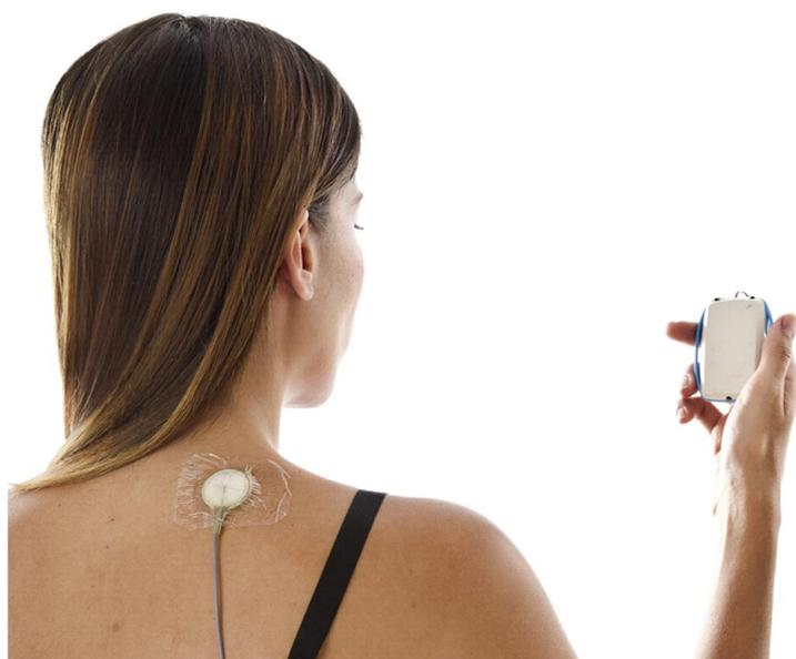
**Figure 1.2:** A wearable self-applied therapeutic ultrasound device [10].
