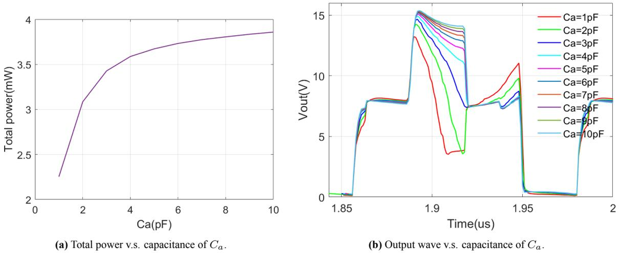
(a) Total power v.s. capacitance of  $C_a$ .(b) Output wave v.s. capacitance of  $C_a$ .**Figure 4.11:** Different capacitance of  $C_a$  with different power consumption and  $V_{out}$ .**Table 4.1:** SELECTIONS OF WIDTHS AND CAPACITANCE IN THE HV DRIVER
