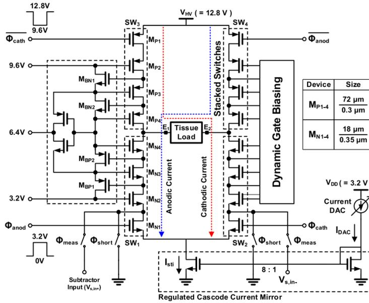
Figure 2.13: Bipolar output current driver with stacked standard CMOS transistors [30].
