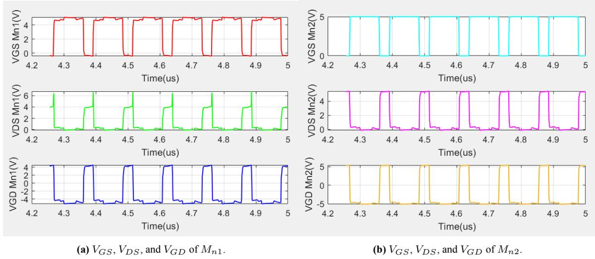
**Figure 4.6:** Voltages between terminals of  $M_{n1}$  and  $M_{n2}$ .
