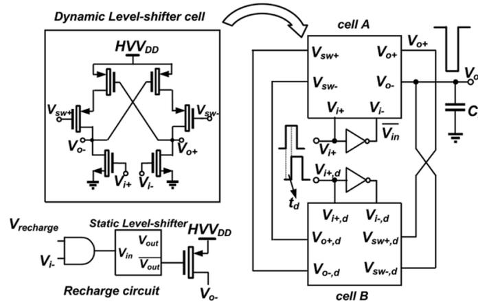
Figure 2.22: Complete architecture of the proposed dynamic level-shifter [36].
