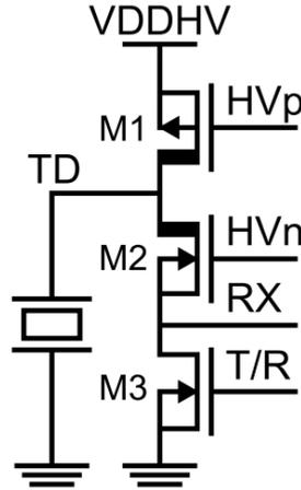
Figure 2.6: Structure of a unipolar pulser [9].
