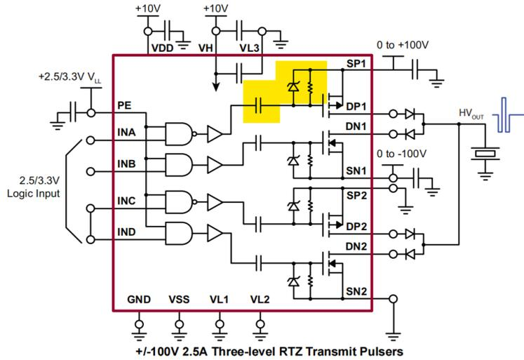
Figure 2.25: Zener-diode level-shifter (yellow part) [36].
