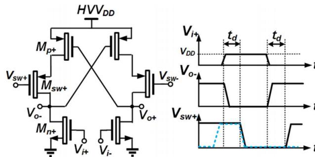
Figure 2.21: Level-shifter with crow-bar current suppression.
