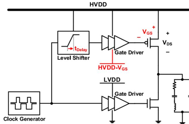
Figure 2.5: Conventional class-D pulser using HV transistors [14].
