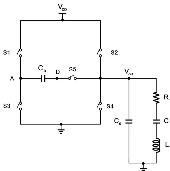
**Figure 3.1:** System-level schematic diagram of the proposed power-efficient HV pulser.
