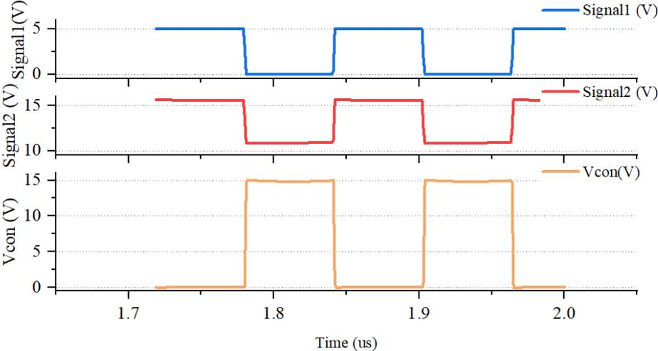
**Figure 4.15:** Transient waveform of control signals and the output voltage of the conventional class-D pulser with 15-V supply voltage.
