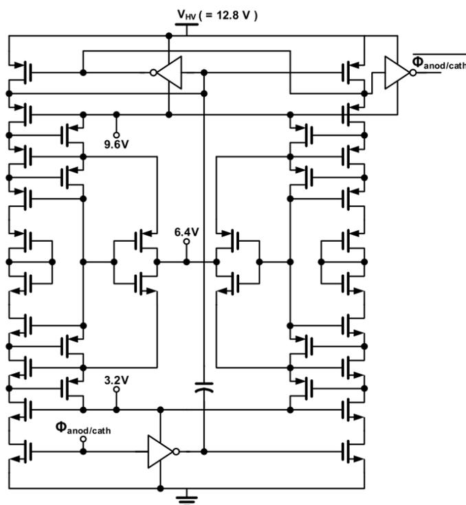
Figure 2.24: A level-shifter using stacked CMOS structure [30].
