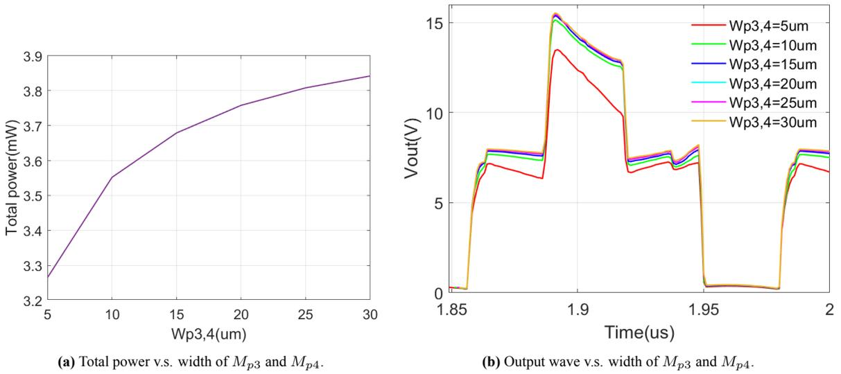
**Figure 4.3:** Different width of  $M_{p3}$  and  $M_{p4}$  with different power consumption and  $V_{out}$ .
