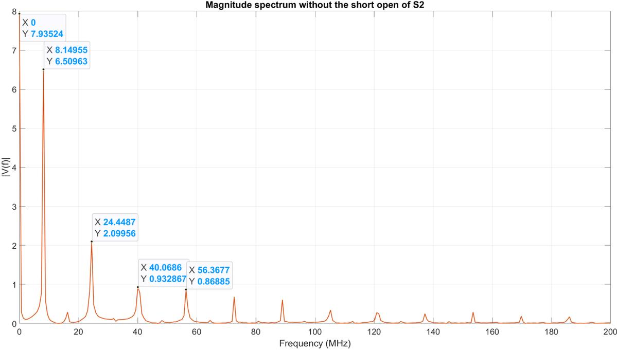
Figure 4.19: Spectrum of the output wave without the short open of S2.
