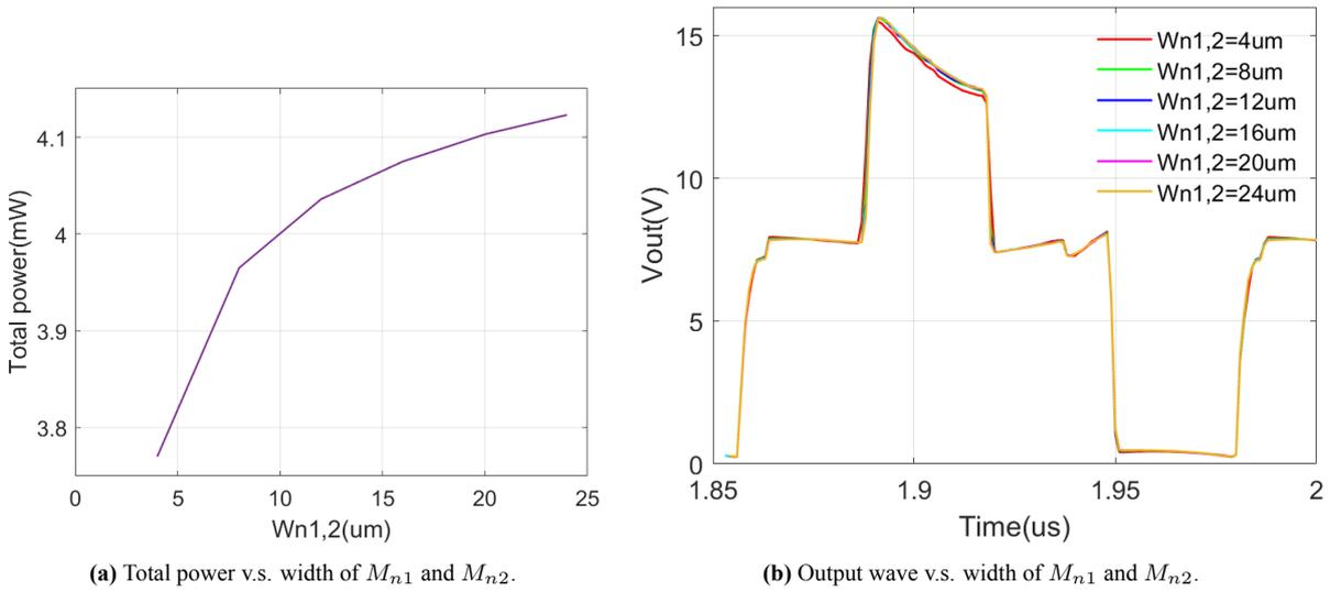
**Figure 4.5:** Different width of  $M_{n1}$  and  $M_{n2}$  with different power consumption and  $V_{out}$ .
