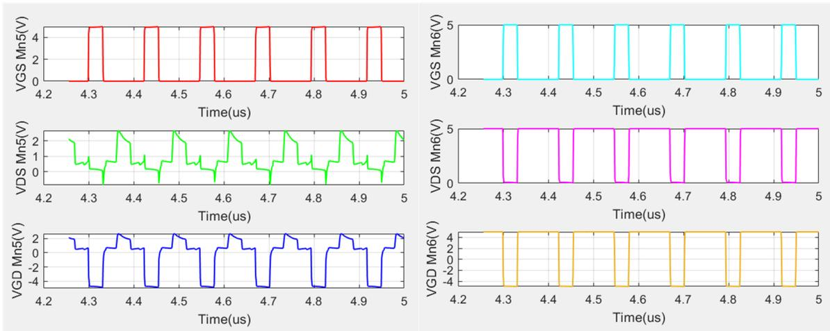
(b)  $V_{GS}$ ,  $V_{DS}$ , and  $V_{GD}$  of  $M_{n5}$  and  $M_{n6}$ .
