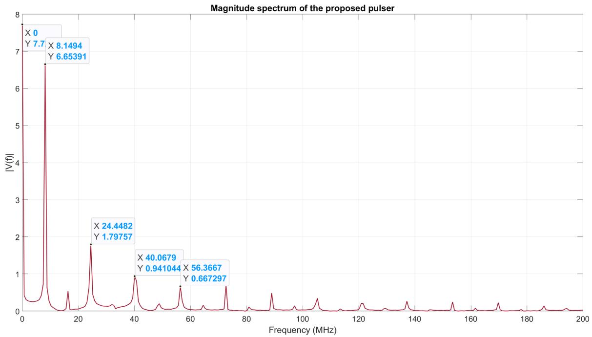
(a) The output wave spectrum of the proposed pulser.
