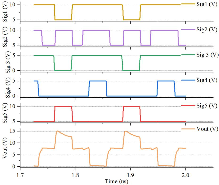
**Figure 4.14:** Transient waveform of control signals and the output voltage wave of the proposed pulser.
