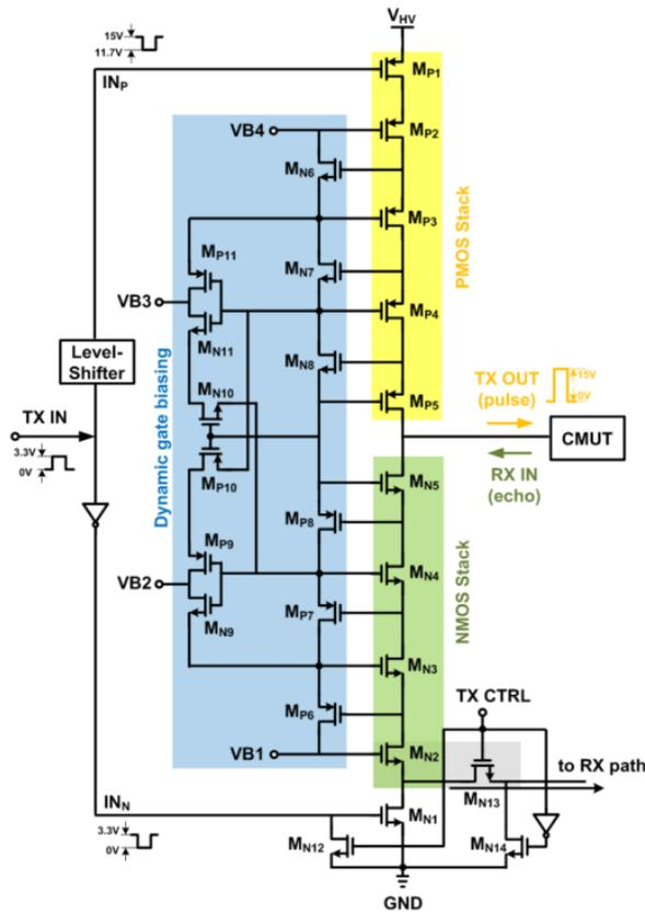
Figure 2.12: Pulser with stacked standard CMOS transistors [29].
