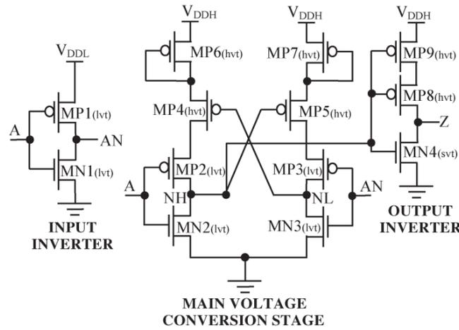
Figure 2.20: Low-power level-shifter [35].
