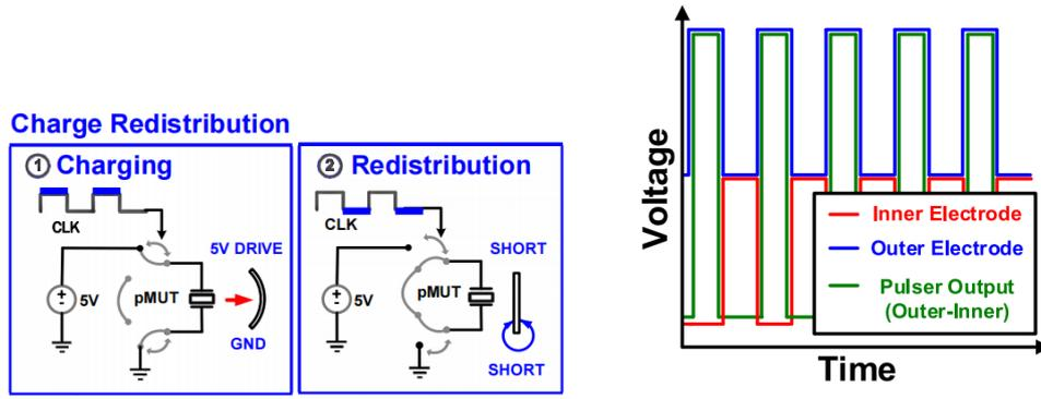
Figure 2.8: (a) Charge redistribution scheme and (b) operation wave forms.
