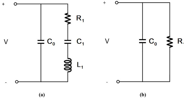
**Figure 2.3:** (a) BVD model for a single resonant frequency PZT transducer (b) Simplified BVD model.
