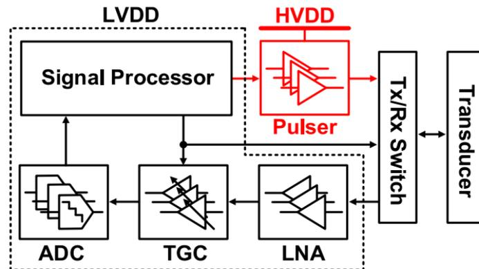
Figure 2.1: Block diagram of the ultrasound transceiver system [14].
