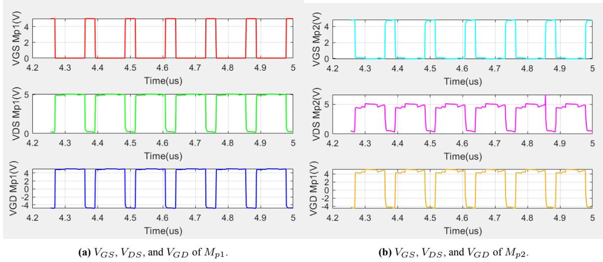
**Figure 4.2:** Voltages between terminals of  $M_{p1}$  and  $M_{p2}$ .
