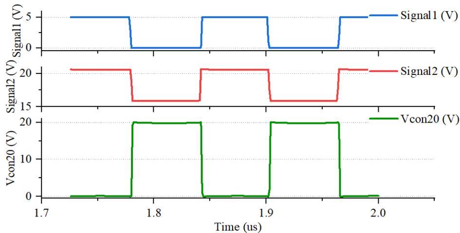
**Figure 4.17:** Transient waveform of control signals and the output voltage of the conventional class-D pulser with 20-V supply voltage.
