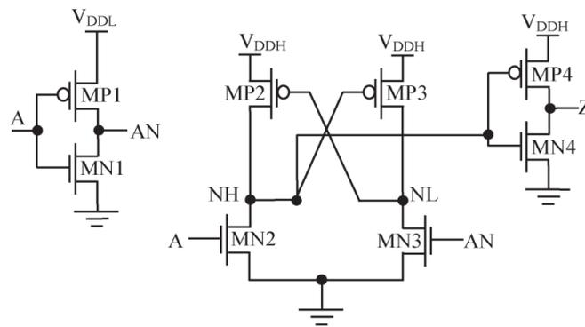
**Figure 2.19:** Conventional DCVS level converter.
