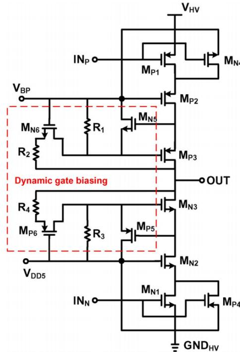
Figure 2.26: HV output driver with gate-biasing part proposed by [38].
