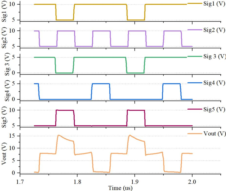
Figure 4.18: Transient waveform of control signals and the output voltage where S2 is not opened during  $\Phi_1$  and  $\Phi_3$ .
