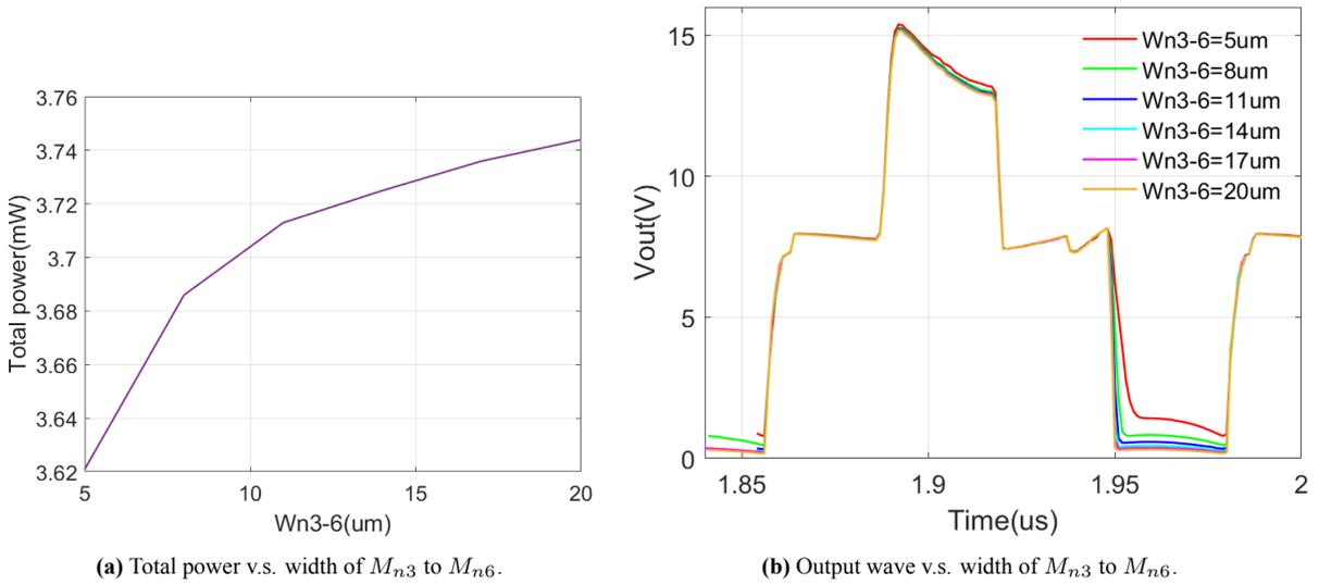
**Figure 4.7:** Different width of  $M_{n3}$  to  $M_{n6}$  with different power consumption and  $V_{out}$ .
