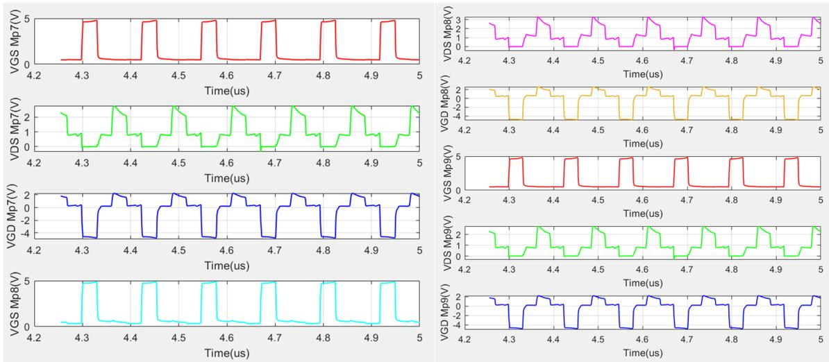
(c)  $V_{GS}$ ,  $V_{DS}$ , and  $V_{GD}$  of  $M_{p7}$  to  $M_{p9}$ .**Figure 4.8:** Voltages between terminals of switch S4.
