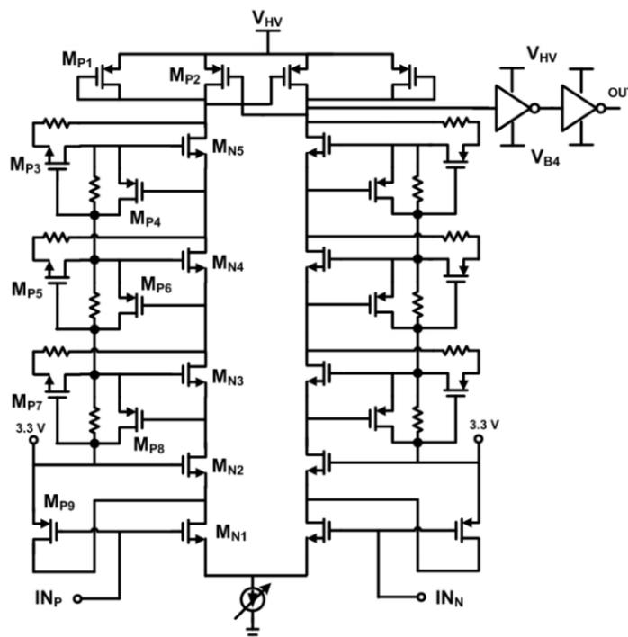
Figure 2.23: A level-shifter using stacked CMOS structure [29].
