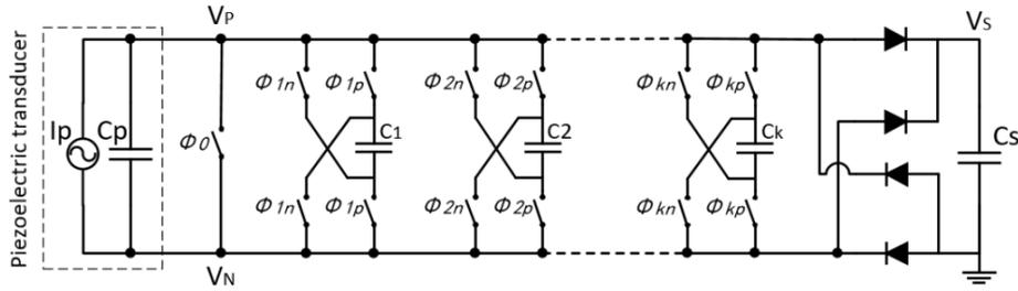
Figure 2.10: SSHC interface circuit with k SCs [27].
