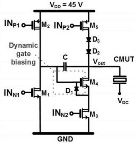
Figure 2.16: Supply-double 3-level pulser.
