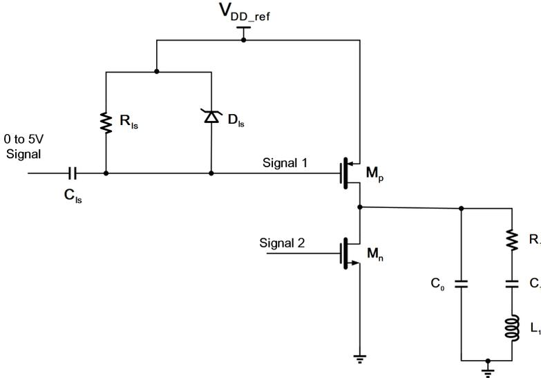
Figure 3.13: The conventional class-D pulser to as the comparison.
