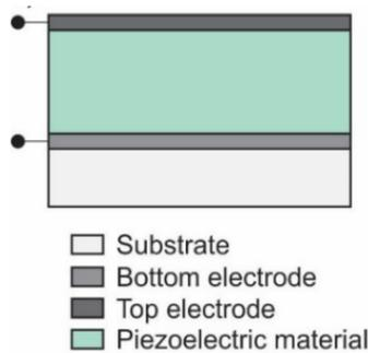
**Figure 2.2:** A bulk piezoelectric material transducer.
