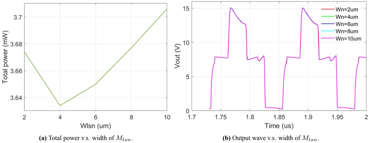
**Figure 4.13:** Different width of  $M_n$  with different power consumption and  $V_{out}$ .
