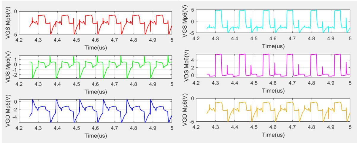
**(a)**  $V_{GS}$ ,  $V_{DS}$ , and  $V_{GD}$  of  $M_{p5}$ .
