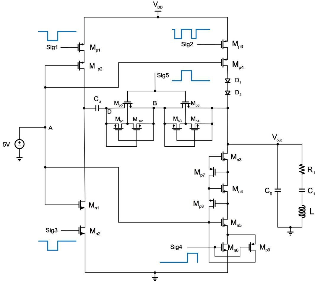
**Figure 3.3:** The output driver implementation.
