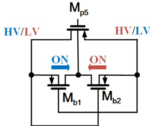
Figure 3.10: The self body biasing circuit.
