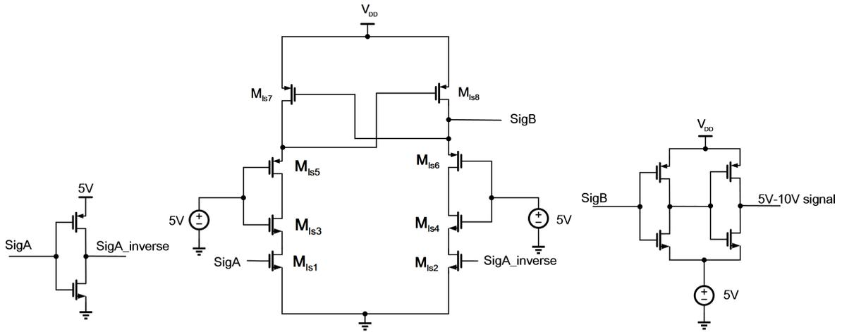
**Figure 3.12:** The level shifter used in the proposed design.
