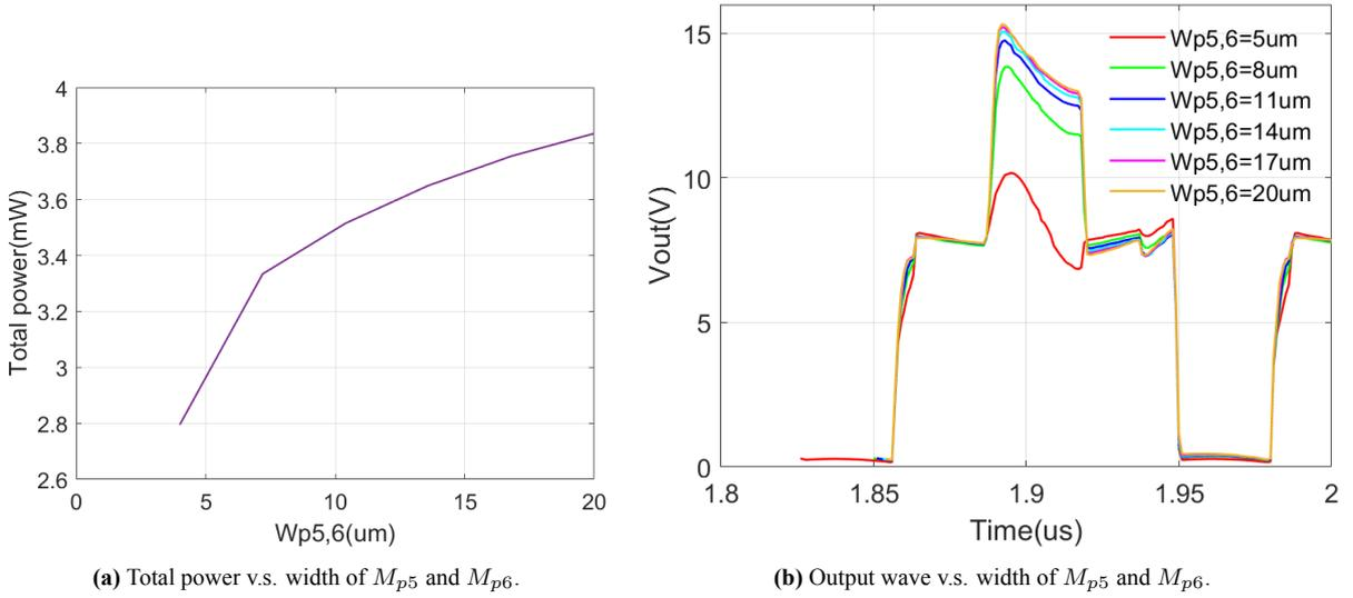
**Figure 4.9:** Different width of  $M_{p5}$  and  $M_{p6}$  with different power consumption and  $V_{out}$ .
