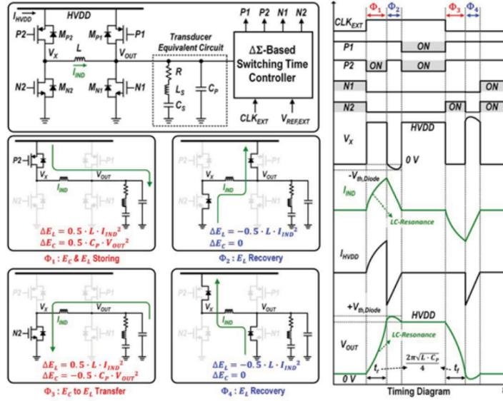
**Figure 2.7:** Operation of the ER pulser in 4 phases- $\Phi_1$ : $E_C$  &  $E_L$  storing,  $\Phi_2$ :  $E_L$  recovery,  $\Phi_3$ : $E_C$  to  $E_L$  transfer,  $\Phi_4$ :  $E_L$  recovery [12].
