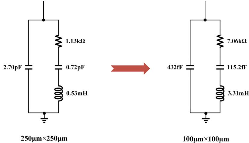
**Figure 3.4:** Scaling the  $100\ \mu\text{m} \times 100\ \mu\text{m}$  PZT transducer element from a  $250\ \mu\text{m} \times 250\ \mu\text{m}$  model.
