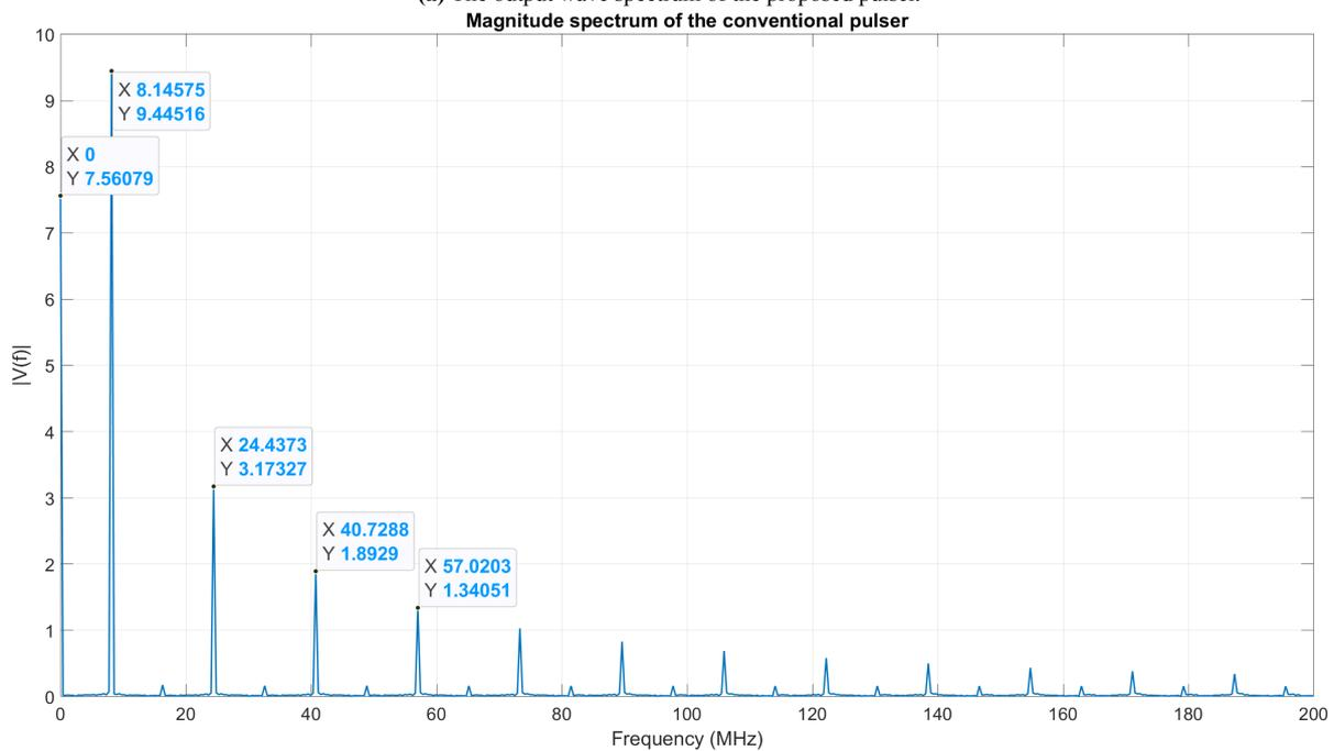
(b) The output wave spectrum of the conventional pulser with 15-V supply voltage.
