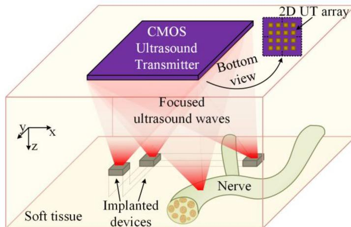
**Figure 2.4:** Conceptual diagram showing operation of a 2D array with 3D control of focal spots [20].
