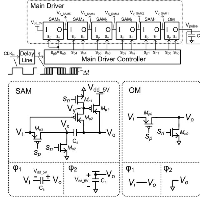
**Figure 2.18:** Circuit schematics of the modulars for the 7-level supply multiplying pulser.
