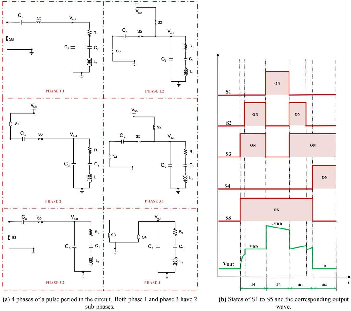
**Figure 3.2:** Operation process of this 3-level pulser.
