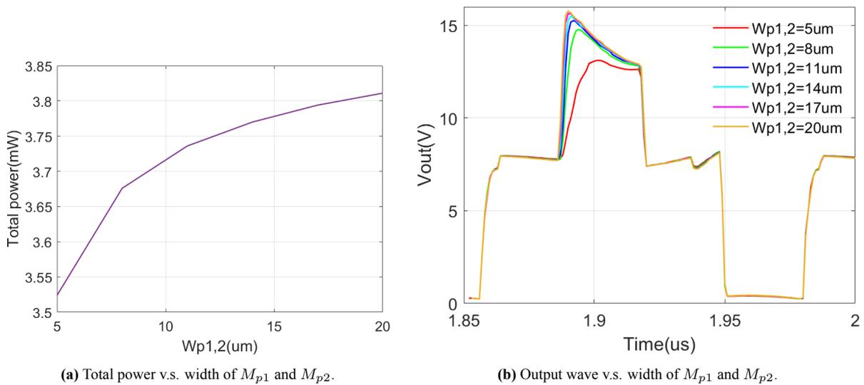
**Figure 4.1:** Different width of  $M_{p1}$  and  $M_{p2}$  with different power consumption and  $V_{out}$ .
