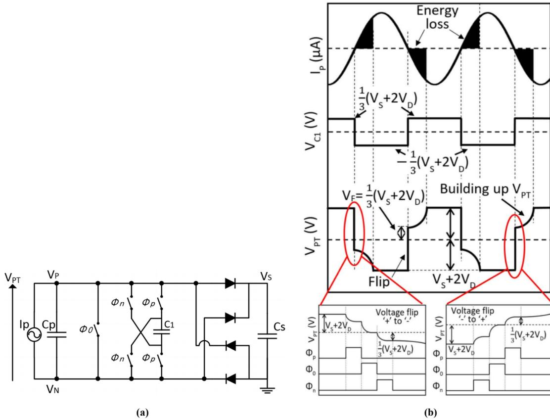
Figure 2.9: (a) SSHC interface circuit with one charge-swap capacitor (b) Waveform [27].
