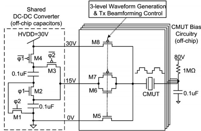
Figure 2.15: A four-channel three-level pulser with the middle-voltage generation [9].
