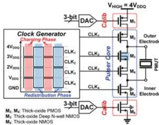
Figure 2.14: Charge redistributed pulser with stacked architecture [31].
