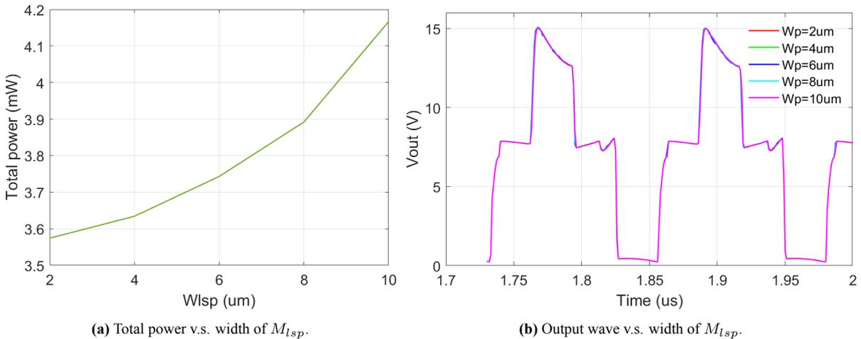
(a) Total power v.s. width of  $M_{lsp}$ .(b) Output wave v.s. width of  $M_{lsp}$ .**Figure 4.12:** Different width of  $M_{lsp}$  with different power consumption and  $V_{out}$ .
