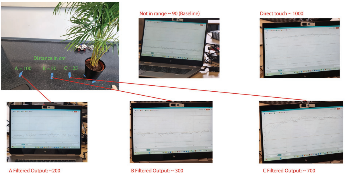
Figure 33. Setup and experiment output overview: Serial plotters showing that the sensor hits the thresholds at different distances.
