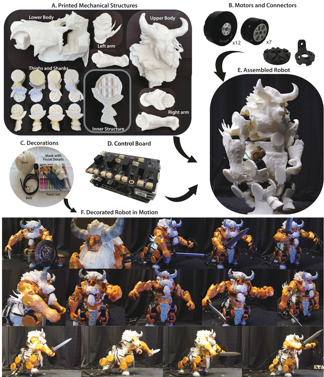
Fig. 2 | Result of a Centaur. A 3D-printed mechanical component of the robot. The initial joint configurations are specified via our UI during preprocessing. Mesh decomposition and the subsequent steps of our system (Fig. 1C) are performed automatically. B Selected motors in the actuator optimization step and the dovetail
