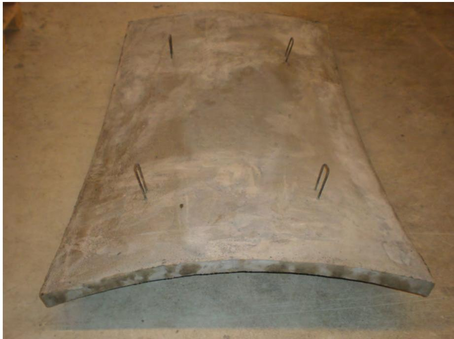
Figure 6: Resulting saddle-shaped panel
