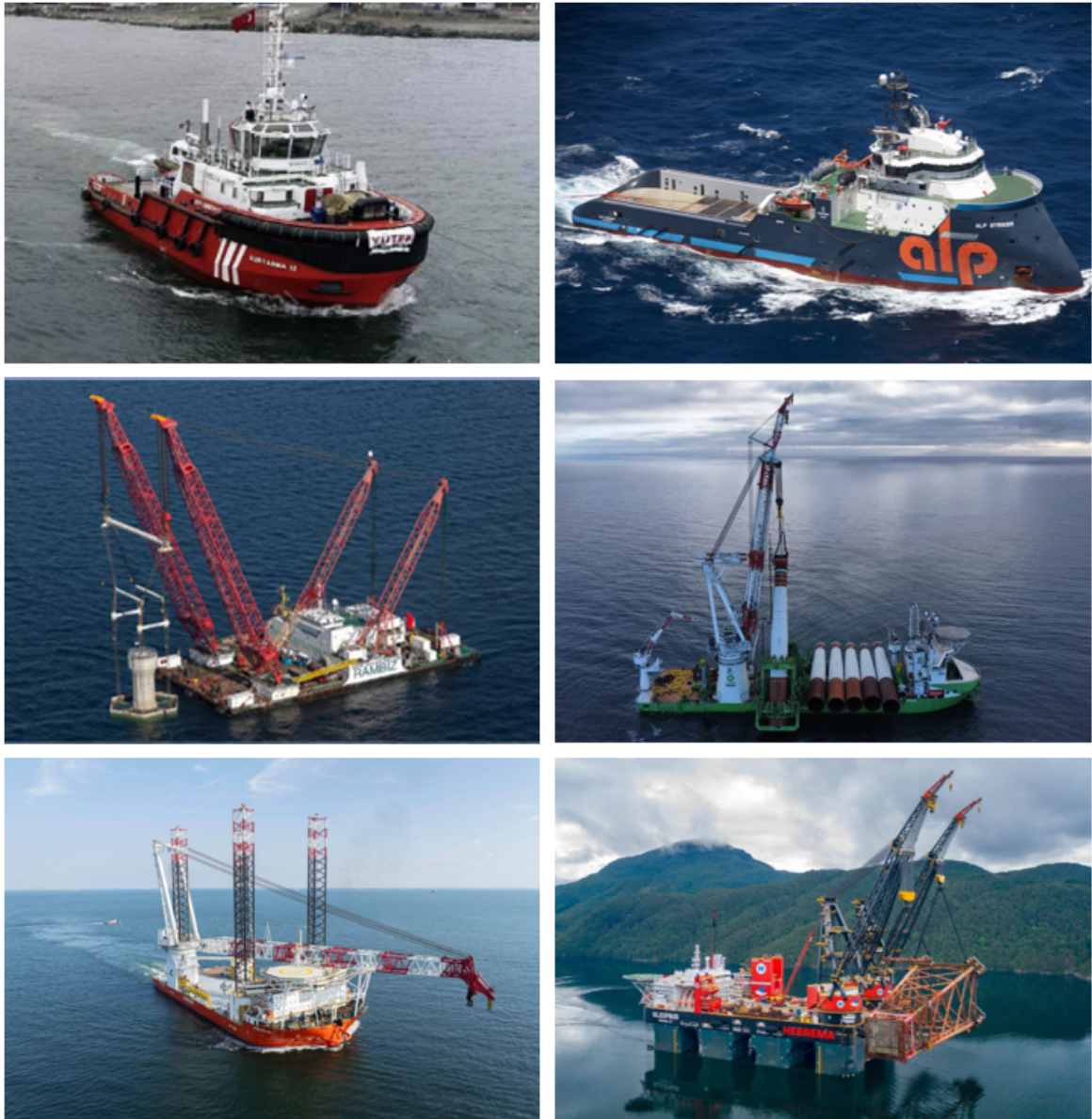
Figure A.1: Vessels operating in the offshore wind industry: Tugboat (upper left) [35], AHTS (upper right) [47], crane barge (middle left) [44], dynamic positioning heavy lift vessel (middle right) [28], jack-up WTIV (lower left) [4] and SSCV (lower right) [9].
