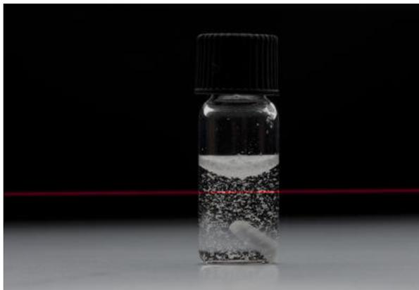
Figure E.4: Measuring turbidity in a glass vial by measuring the transmissivity of a red laser [119].
