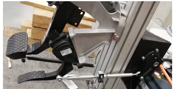
Figure 2: The active accelerator and brake pedals, in the front and back respectively. The pedals are both connected to a control loader via a metal rod. Halfway the metal rod, a force cell is placed.
