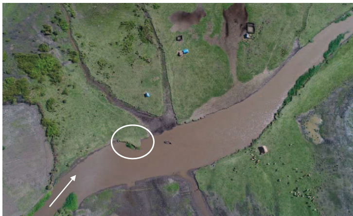
Fig. 1. Lower course of the Mara River (Tanzania). The rock outcrop protruding from the left bank, in the white circle, acts as an isolated groyne and produces opposite bank erosion (visible bank failures). Flow from left to right. UAV image, courtesy of Francesco Bregoli.
