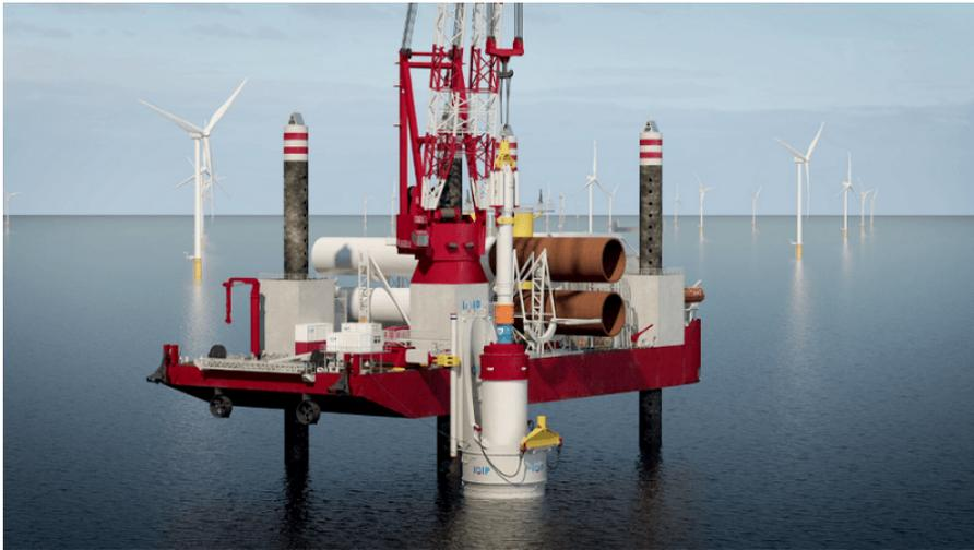
**Figure 2.2:** Integration of IQIP PULSE system in offshore monopile installation (IQIP, 2020).
