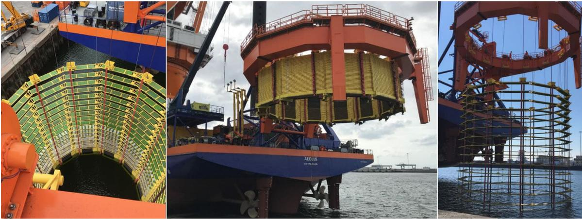
Figure 2.6: AdBm system with Helmholtz resonators for underwater noise mitigation (AdBm Technologies, 2024).
