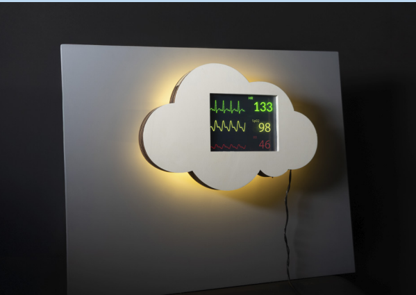
Figure 4.18: Physical prototype of the Care Cloud when window is transparent, and monitor is visible.
