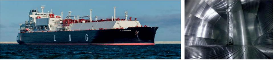
Figure 1.1: LNG vessel (left) [obtained from Mokhatab *et al.*, Handbook of Liquefied Natural Gas, 2014], and cargo containment system (right) [obtained from GTT.fr].
