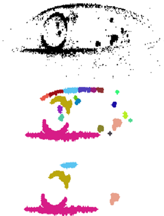
Figure 2.5: An example of adhered eye parts. The pupil arc in red is mixed with the eyelid. The method cannot split the adhesion.
