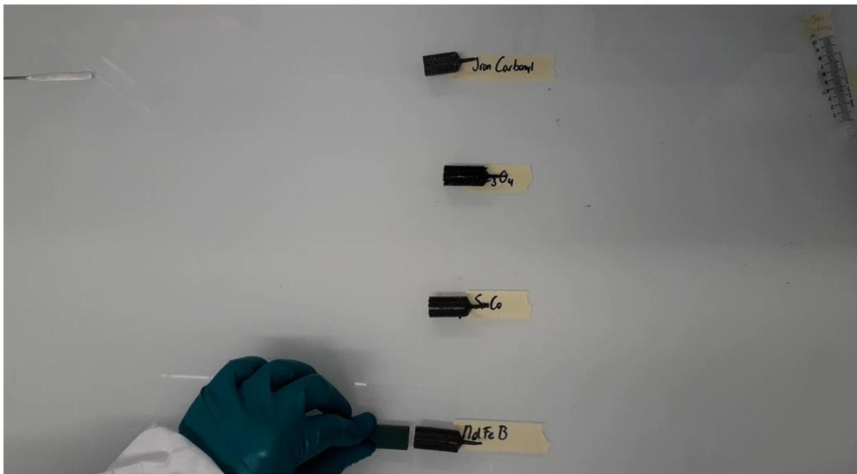
Figure 1 *NdFeB* particles are not attracted by the magnetic field, which was the case for this orientation of the magnet in experiment 1
