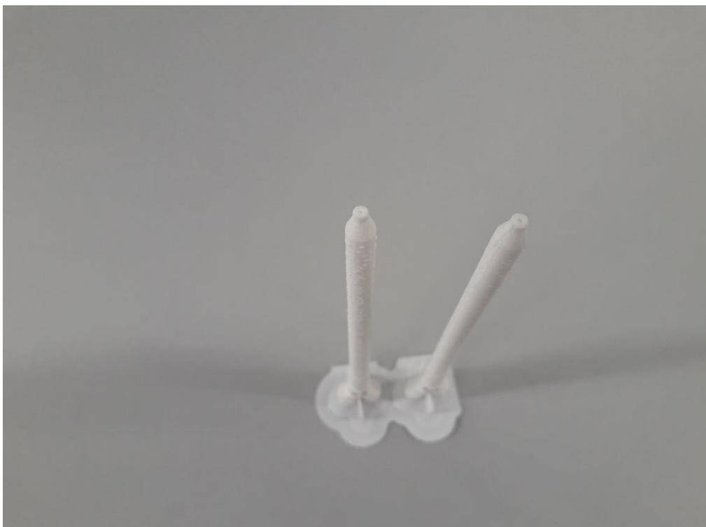
*Figure 5 Printed static mixing nozzles third attempt open nozzles with a diameter of 0.4 mm*
