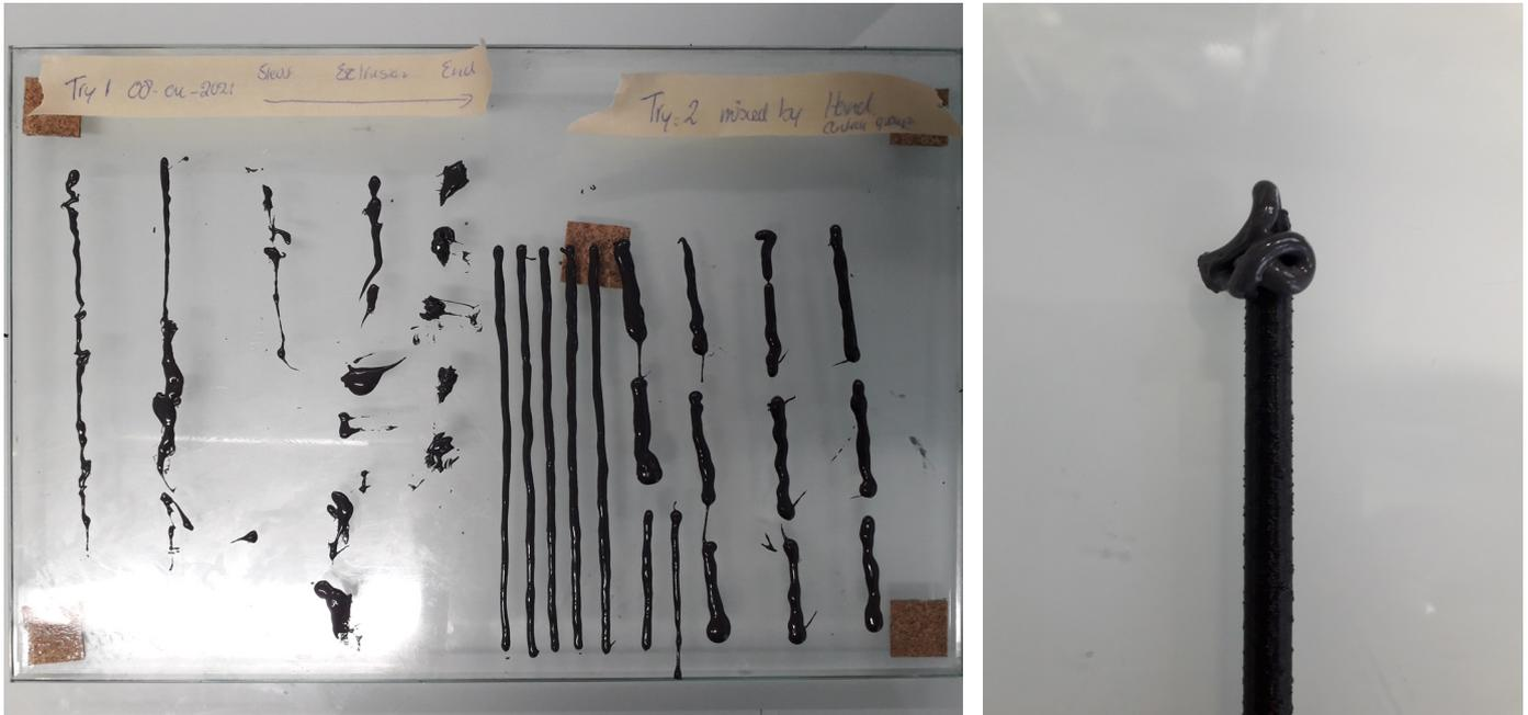
**Figure 3.32:** Extruded static mixing nozzle ink and manually mixed ink, both cured. The ink that cured inside the nozzle.
