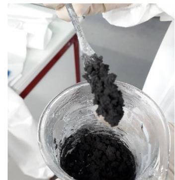
Figure 5 Ecoflex part B mixed with iron powder, Ecoflex part A and fumed silica
