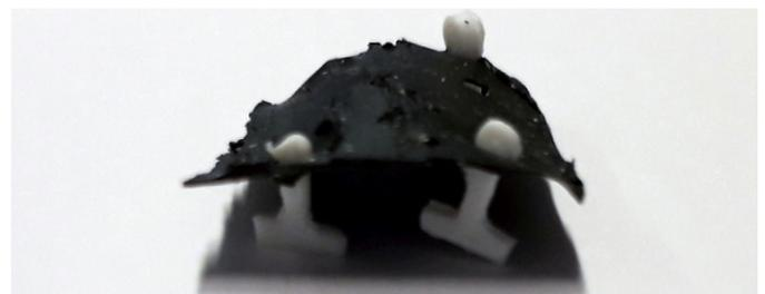
**Figure 4.29:** Prototype of the designed connectors. The best size had a thickness of 0.8 mm for the straight parts and a diameter of 1.6 mm for the circle on top.
