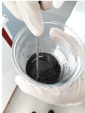
Figure 3 Ecoflex part B mixed with iron powder
