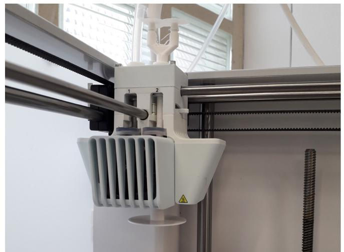
**Figure 3.40:** (top) The thread at the end of the static mixing nozzle. (bottom) The extended static mixing nozzle in the printer head with a prototype for the electromagnet spindle turned on.
