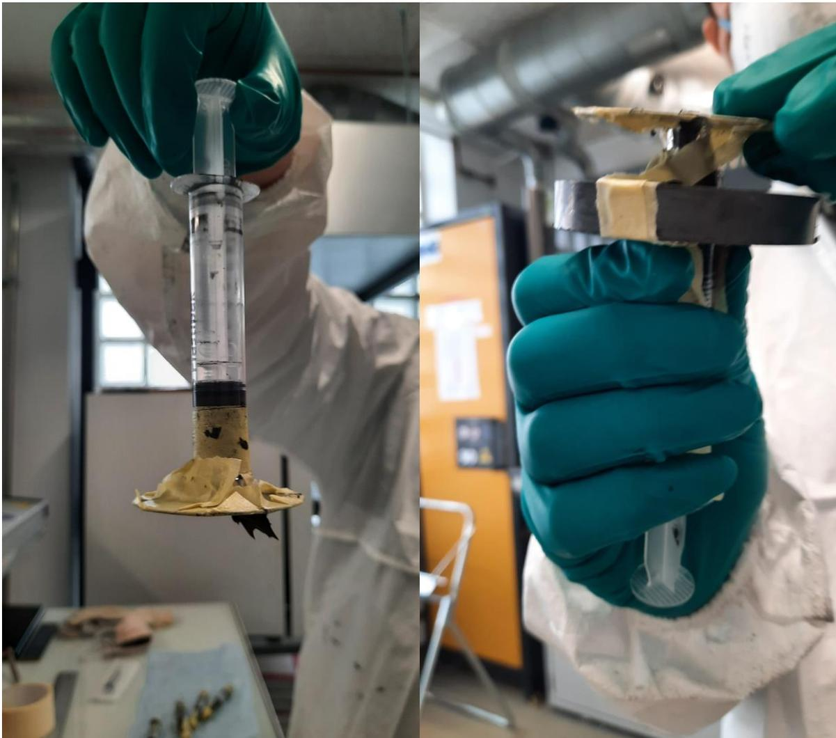
Figure 4 Syringes with mixed ink and a ring magnet at the nozzle. (left) Small NdFeB magnet at the nozzle. (right) Larger ferrite magnet, further up the syringe to prevent the magnetic field from pulling the extruded ink of the glass plate.
