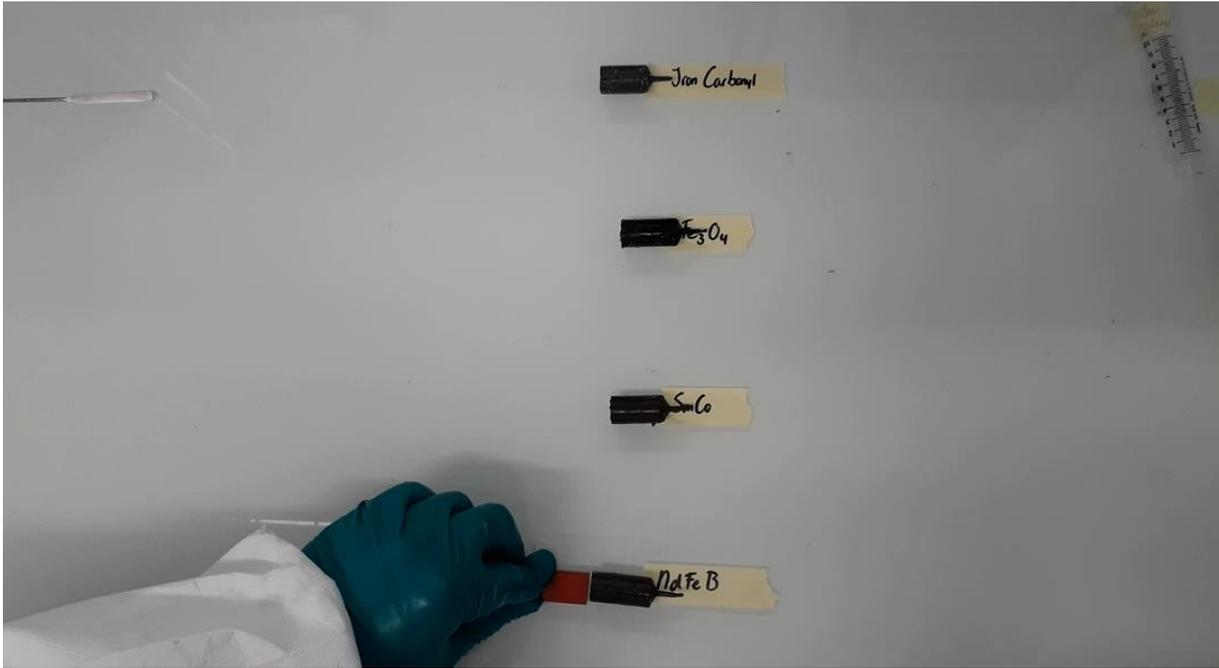
Figure 2 The NdFeB sample is not pushed away as was the case in magnetizer experiment 1 with this orientation of the magnet
