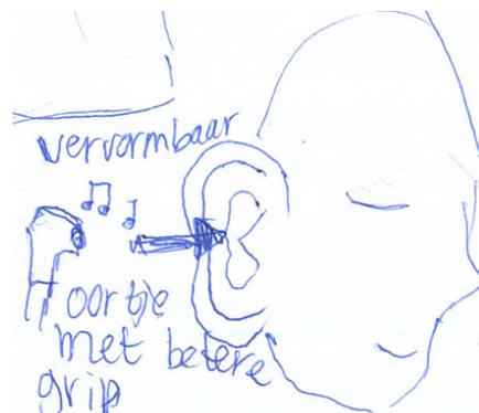
**Figure 4.6:** The magnetic field activates the magnetic soft material in the embodiment of earphones, to make the embodiment adjust to the shape of the ear of the user
