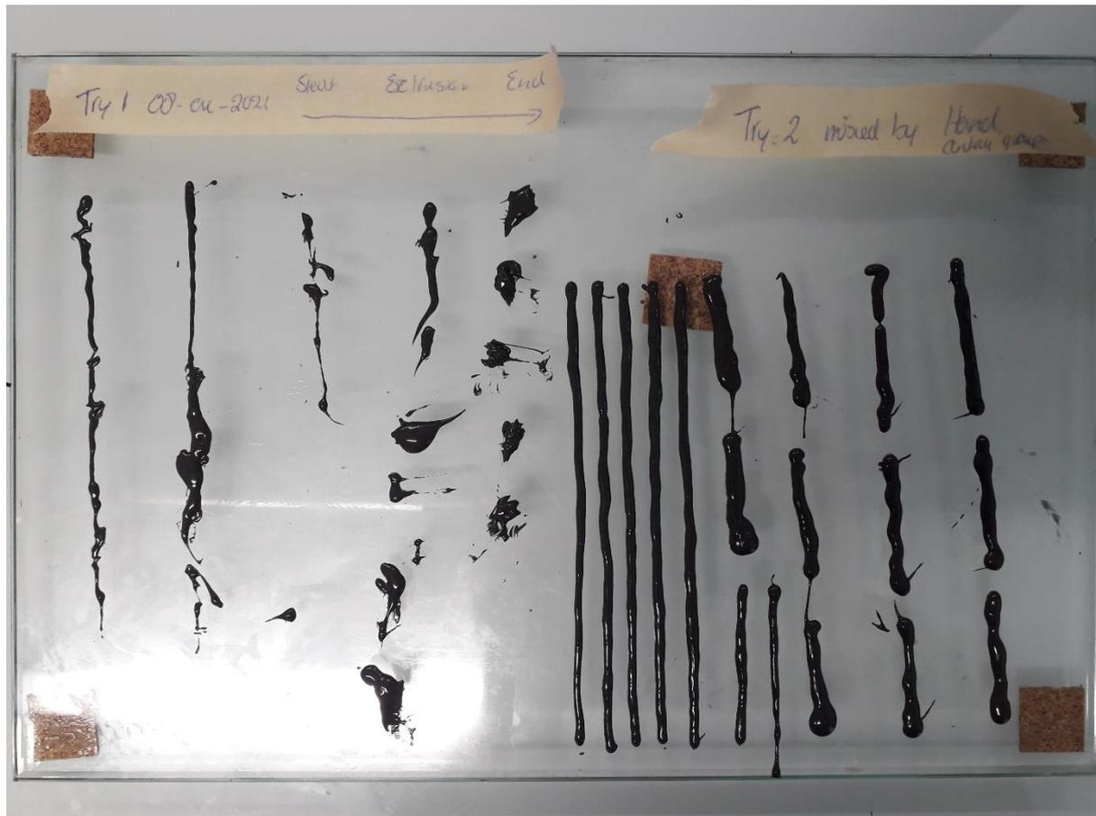
Figure 1 Cured ink. On the left: Cured ink mixed and extruded by the static mixing nozzle. On the right: ink mixed by hand and extruded with the help of a syringe (control group)
