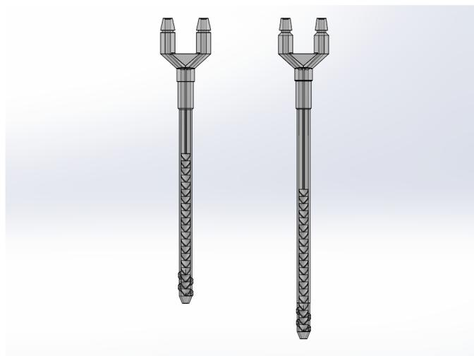
**Figure 3.39:** The original static mixing nozzle length and the extended static mixing nozzle. The extension was made in the part where both ink components are still separate to not add extra additional needed force in the system.
