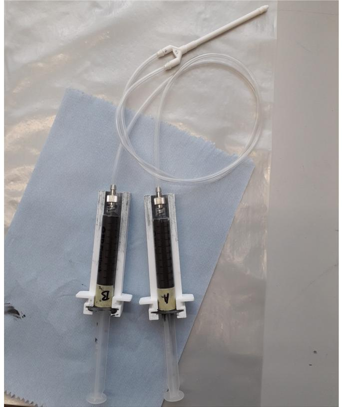
**Figure F.2:** The ink guiding system: conversion pieces, 10 mL syringes, Luer lock connections, tubes, static mixing nozzle
