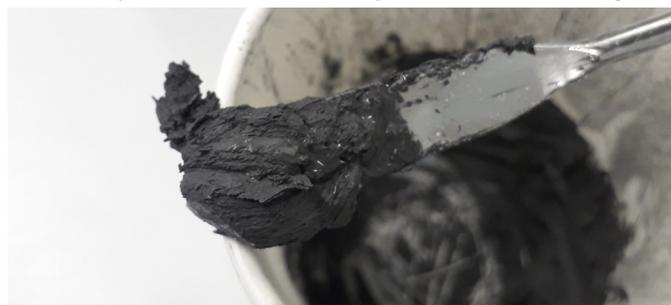
**Figure 3.8:** The smoother, less viscous ink with the 1:1 ratio from experiment 2
