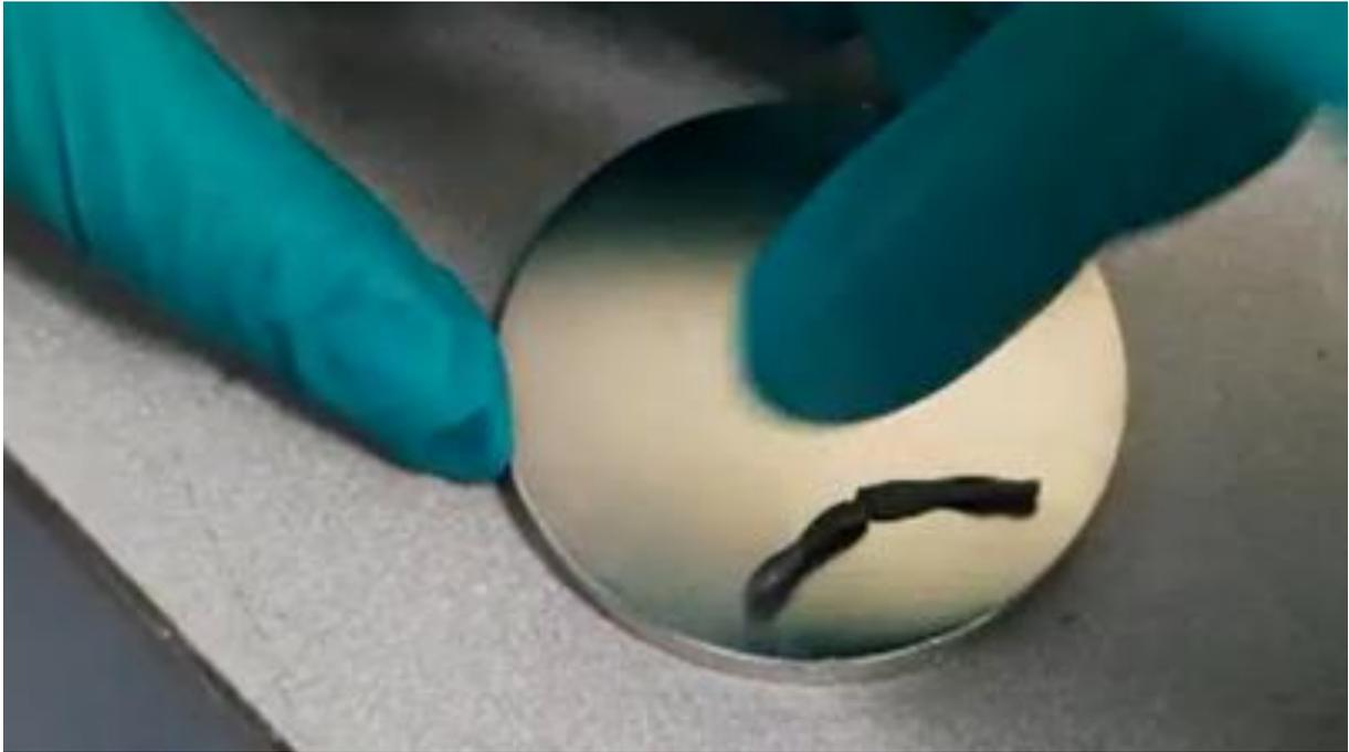
Figure 12 The ends of the extruded strip curl up in the magnetic field of the Neodymium magnet
