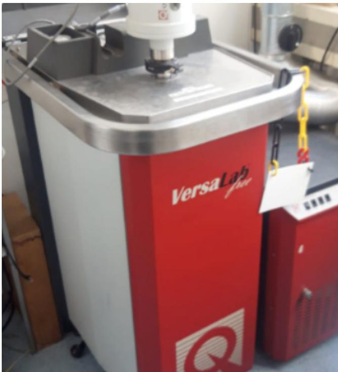
**Figure 3.13:** VersaLab used for magnetizing the ink
