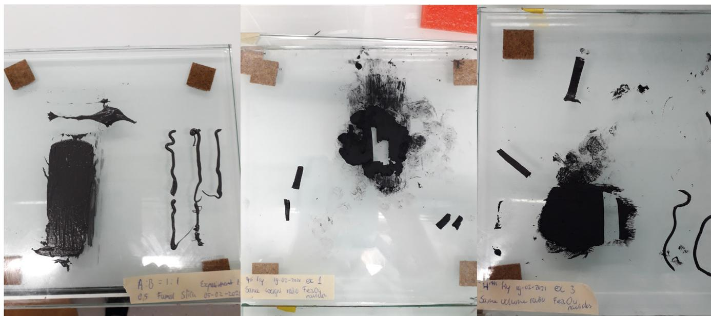
**Figure 3.25:** On the left is the Fe50%SiO<sub>n</sub>M ink with iron carbonyl particles on which the other two inks are based. In the middle is the Fe50%SiO<sub>n</sub>M ink of which the iron carbonyl particles are converted to Fe<sub>3</sub>O<sub>4</sub> particles by wt%. On the right is the Fe50%SiO<sub>n</sub>M ink of which the iron carbonyl particles are converted to Fe<sub>3</sub>O<sub>4</sub> particles by vol%.
