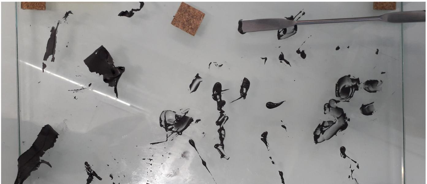
**Figure 3.33:** Ink out of the static mixing nozzle that after the curing time had not cured
