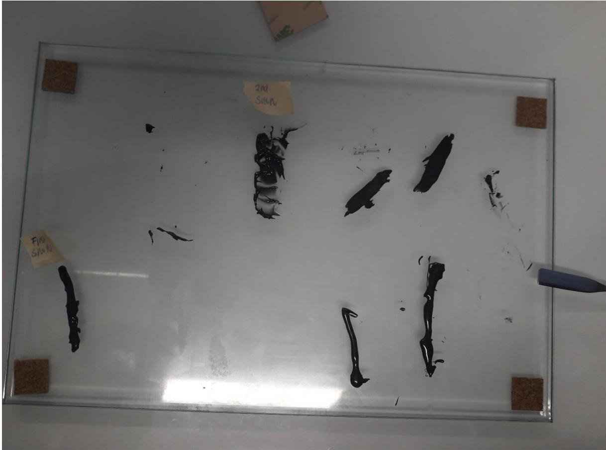
Figure 4 Cured ink. Left: cured ink static mixing nozzle v2. Right; cured ink static mixing nozzle v1.
