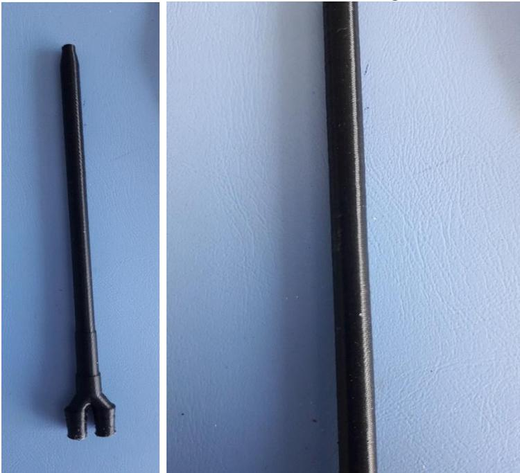
Figure 1 Smoother print static mixing nozzle v2
