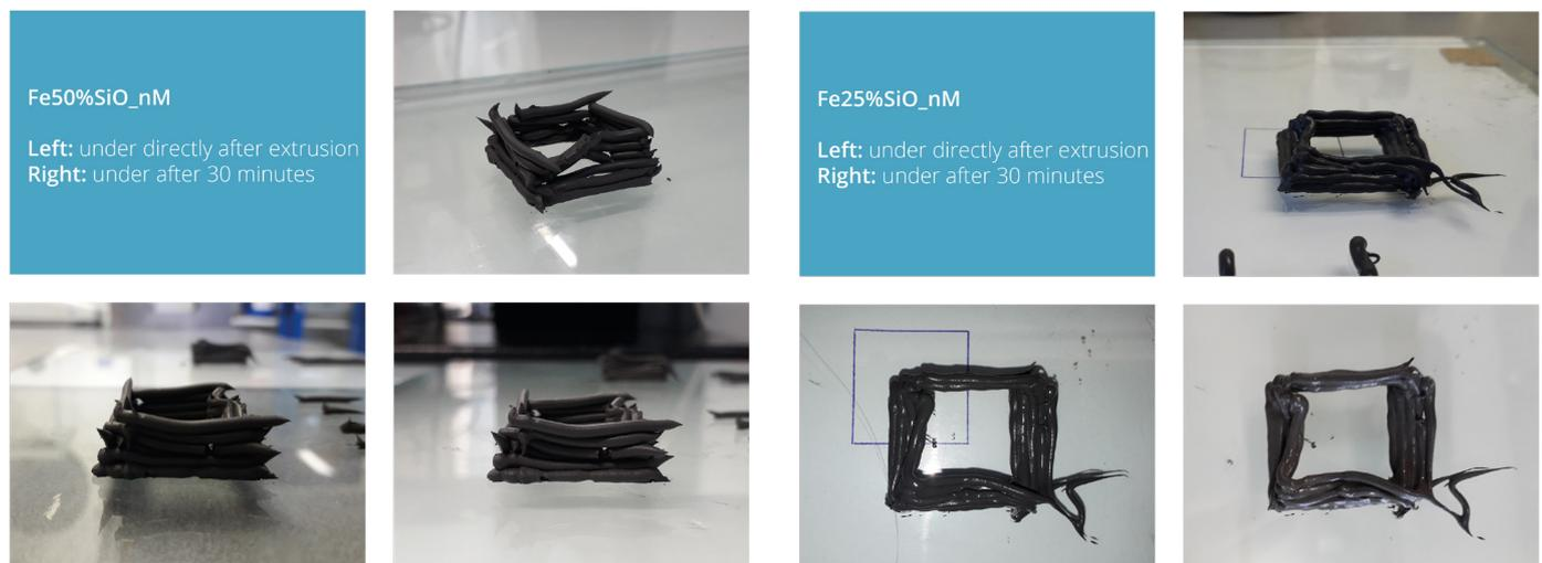
**Figure 3.24:** Fe50%SiO<sub>n</sub>M has a higher viscosity than Fe25%SiO<sub>n</sub>M and is better at holding its shape. The holes present just after the ink was extruded were still present after more than 30 minutes of waiting. The Fe25%SiO<sub>n</sub>M collapsed during the extrusion by hand (which could be a human error), and the extruded lines blended more into each other than the Fe50%SiO<sub>n</sub>M.
