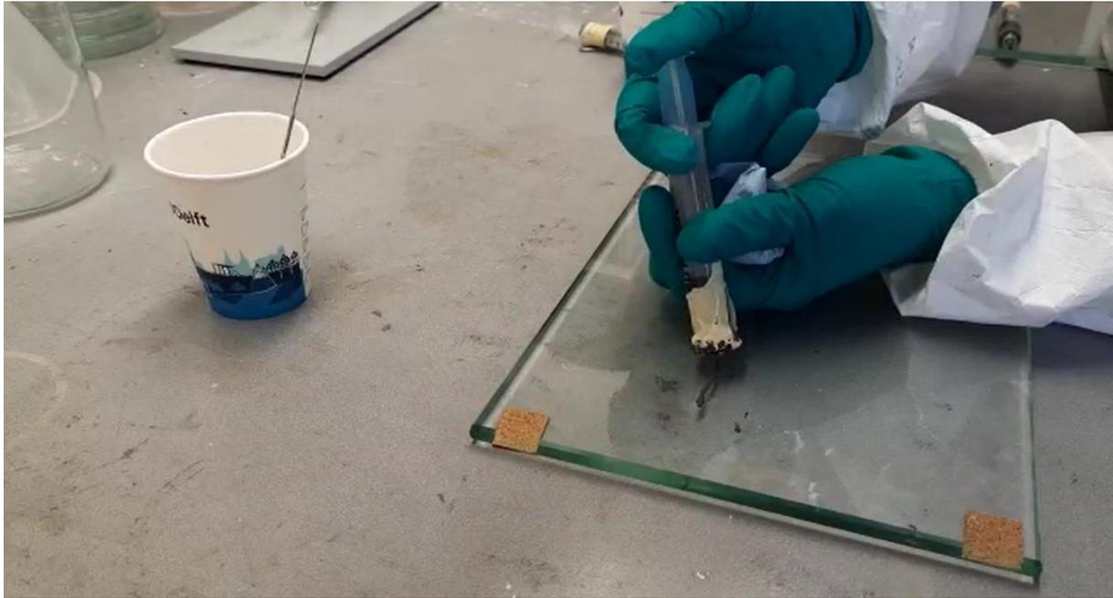
Figure 5 Extrusion of the mixed magnetized ink through the syringe with the mounted on ring magnet
