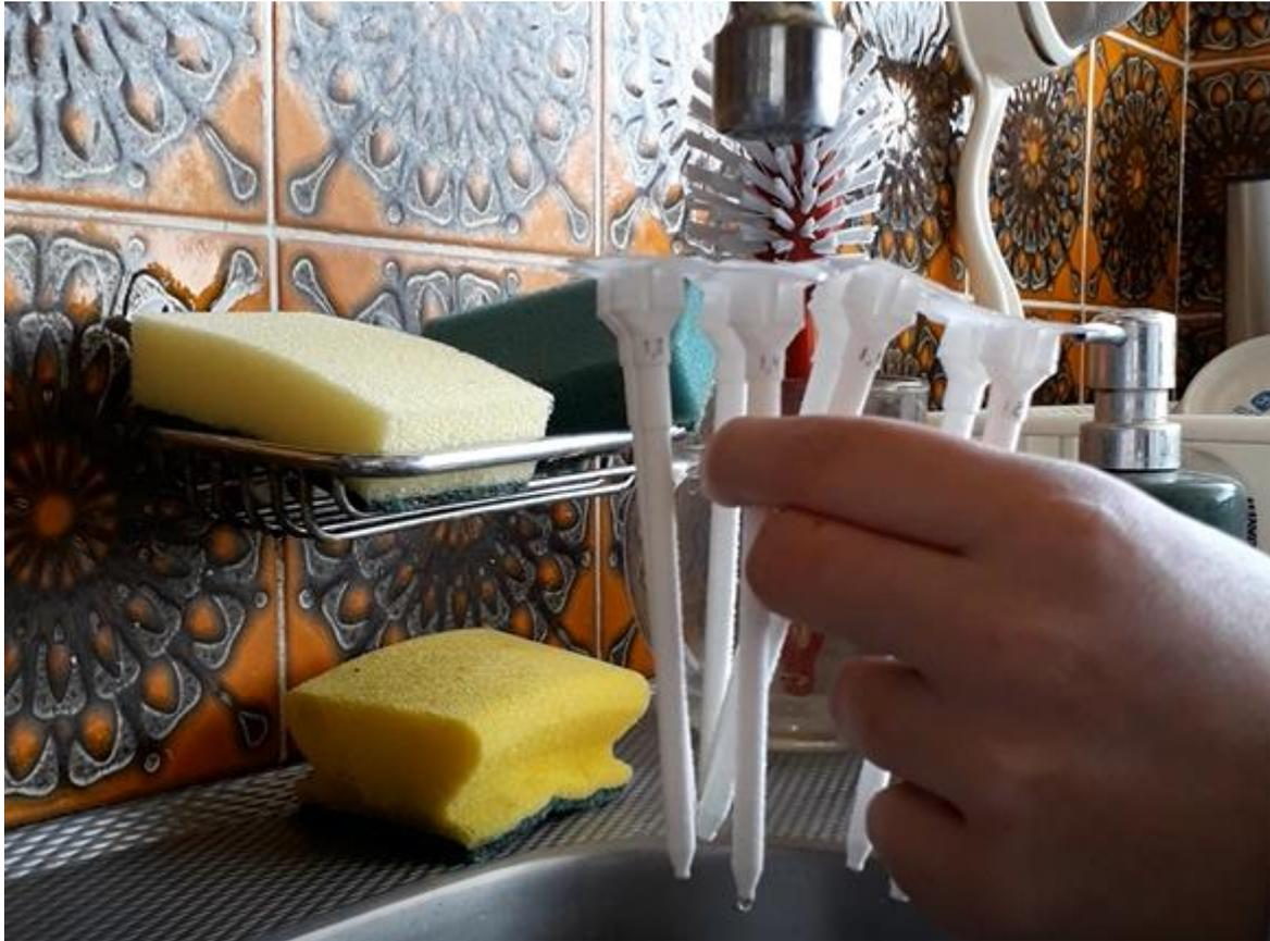
*Figure 7 Test if the static mixing nozzles are hollow by running water through them*
