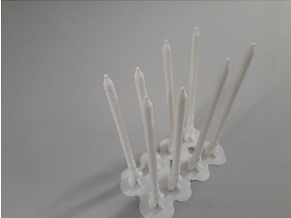
*Figure 4 Printed static mixing nozzles first attempt, closed nozzles*
