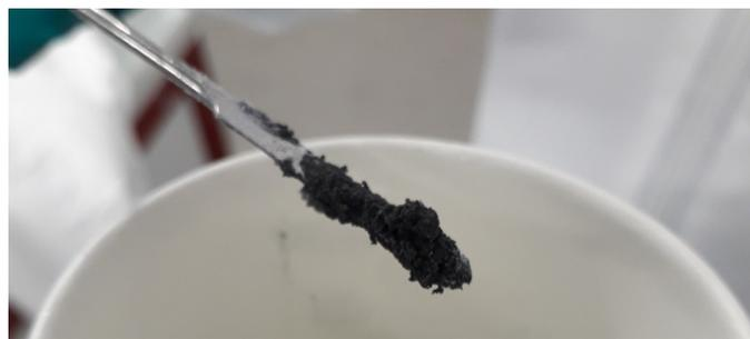
**Figure 3.7:** The grainy texture of the more viscous ink with the altered MIT ratio (B>A) from experiments 1 and 2
