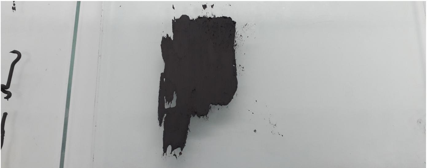
**Figure 3.9:** The ink with the 2A:1B ratio from experiment 3 which was too viscous to extrude through a 10 ml syringe
