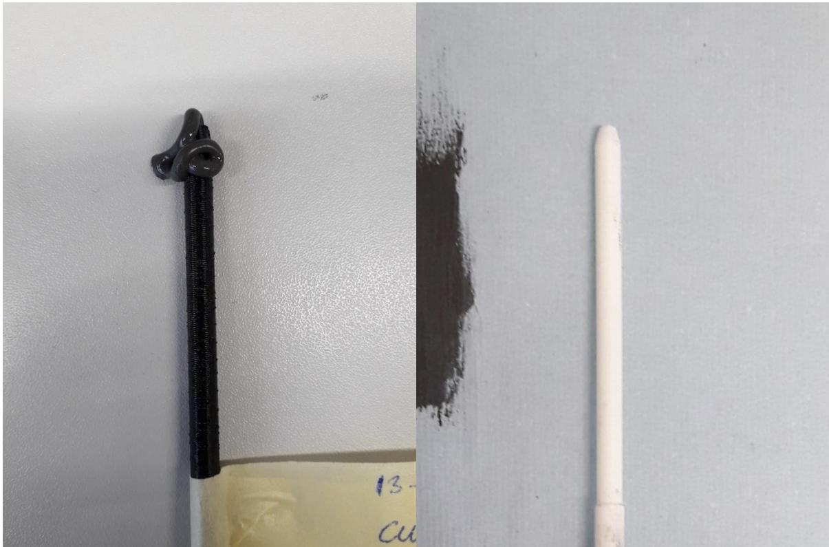
Ink curing after extrusion through the static mixing nozzle (static mixing nozzle test)
