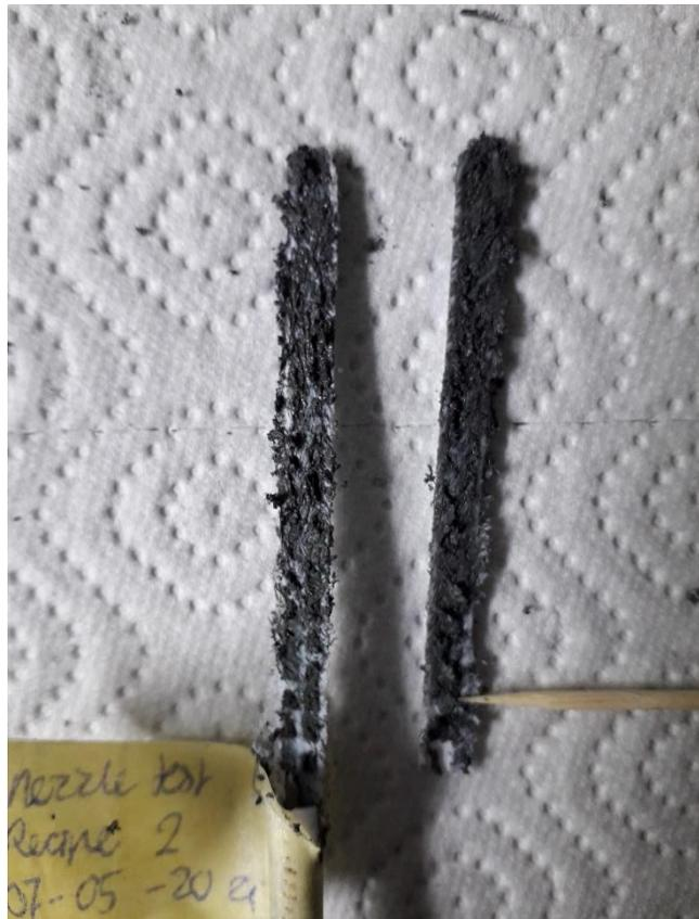
Figure 2 Sawn open static mixing nozzle v1 with T6E4 ink
