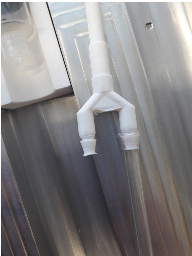
**Figure 3.36:** The new connections at the static mixing nozzle to secure the tubes
