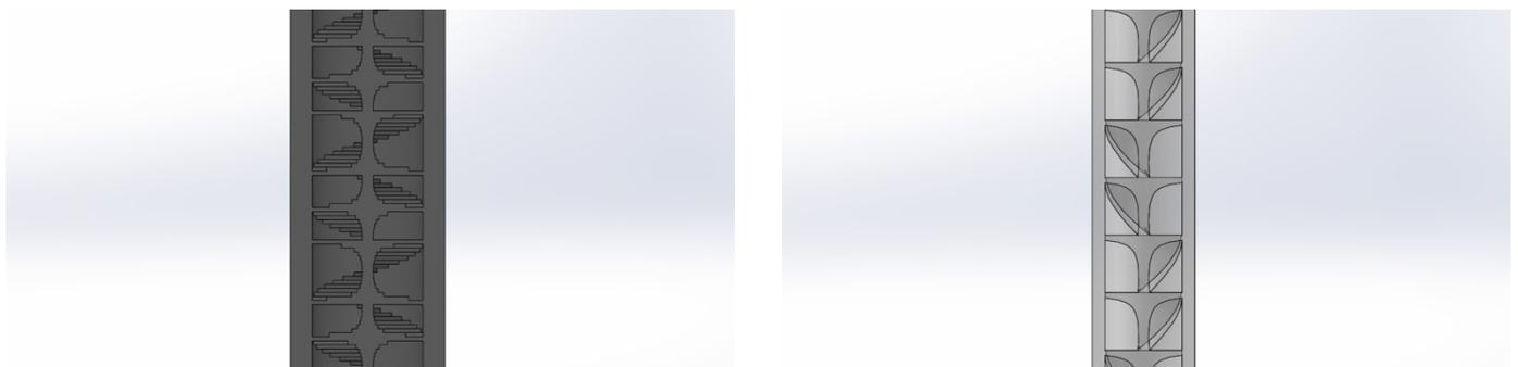
**Figure 3.31:** The mixing mechanism inside static mixing nozzle v2 (1 left, 1 right) and v1 (2 left, 2 right)
