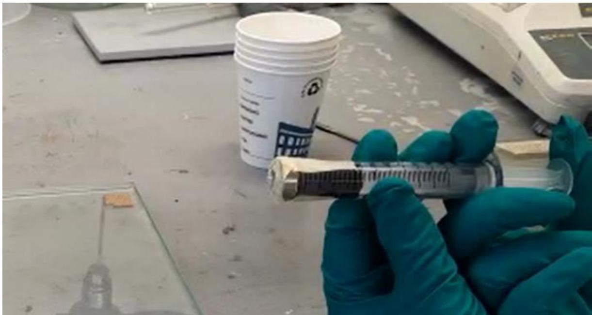
Figure 4 Syringe with mixed ink and a ring magnet at the nozzle
