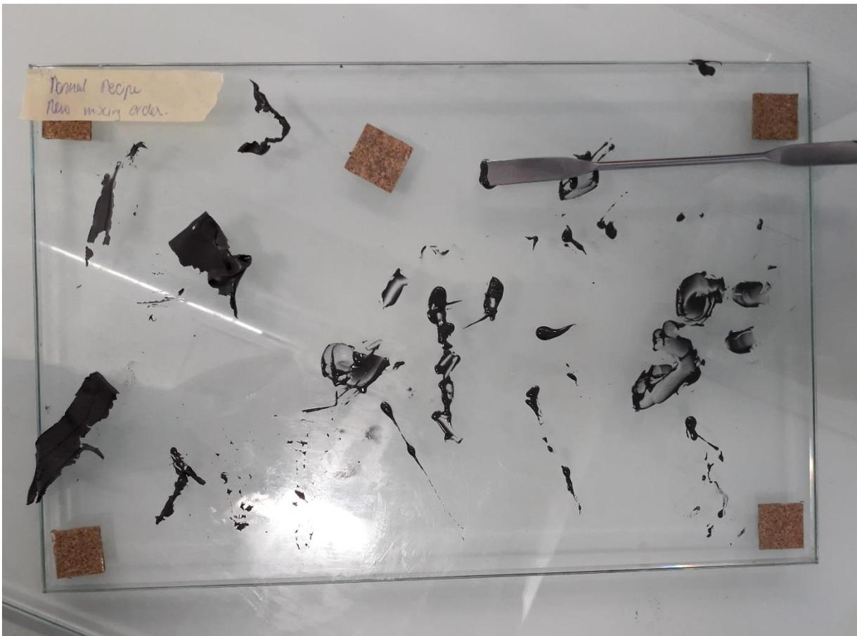
Figure 10 Glass plate with on the left the cured manually mixed material with the new mixing order and on the right the uncured ink of the third try that got extruded through the static mixing nozzle.
