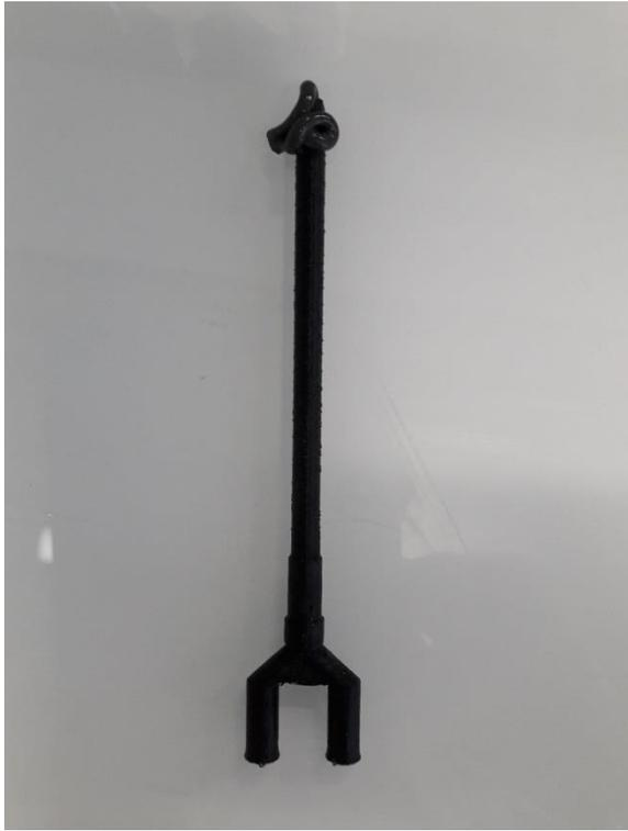
The T7E1 was cured after it was extruded and mixed through the static mixing nozzle. The extruded ink had already a bit of print stability because the extruded ink has a more defined extruded shape, and the ink did not blend together in an unrecognizable shape of ink.
