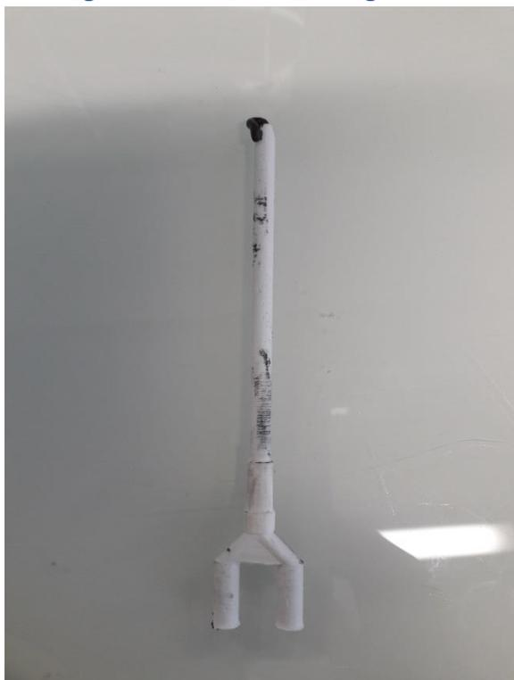
The T6E3 NdFeB ink was cured after it was extruded and mixed through the static mixing nozzle.
