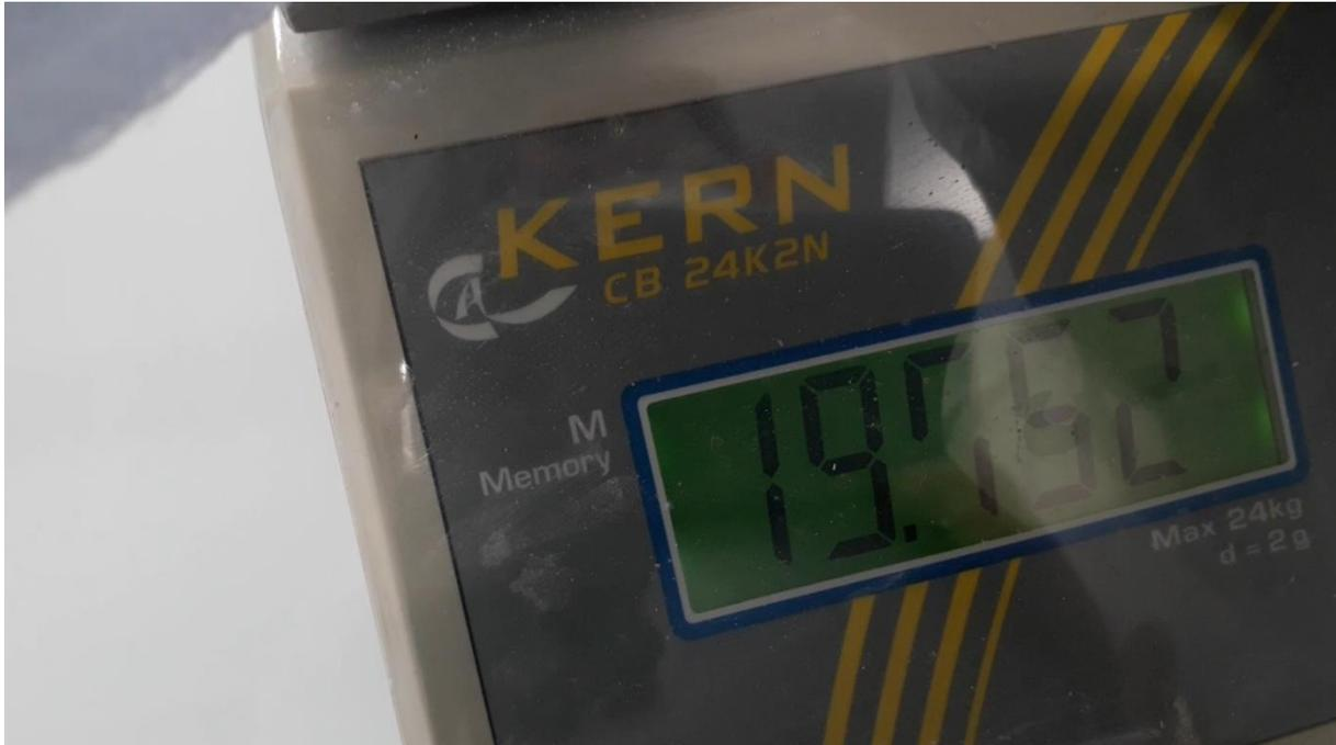
Figure 2 Maximum amount of Kg during the extrusion through static mixing nozzle v2
