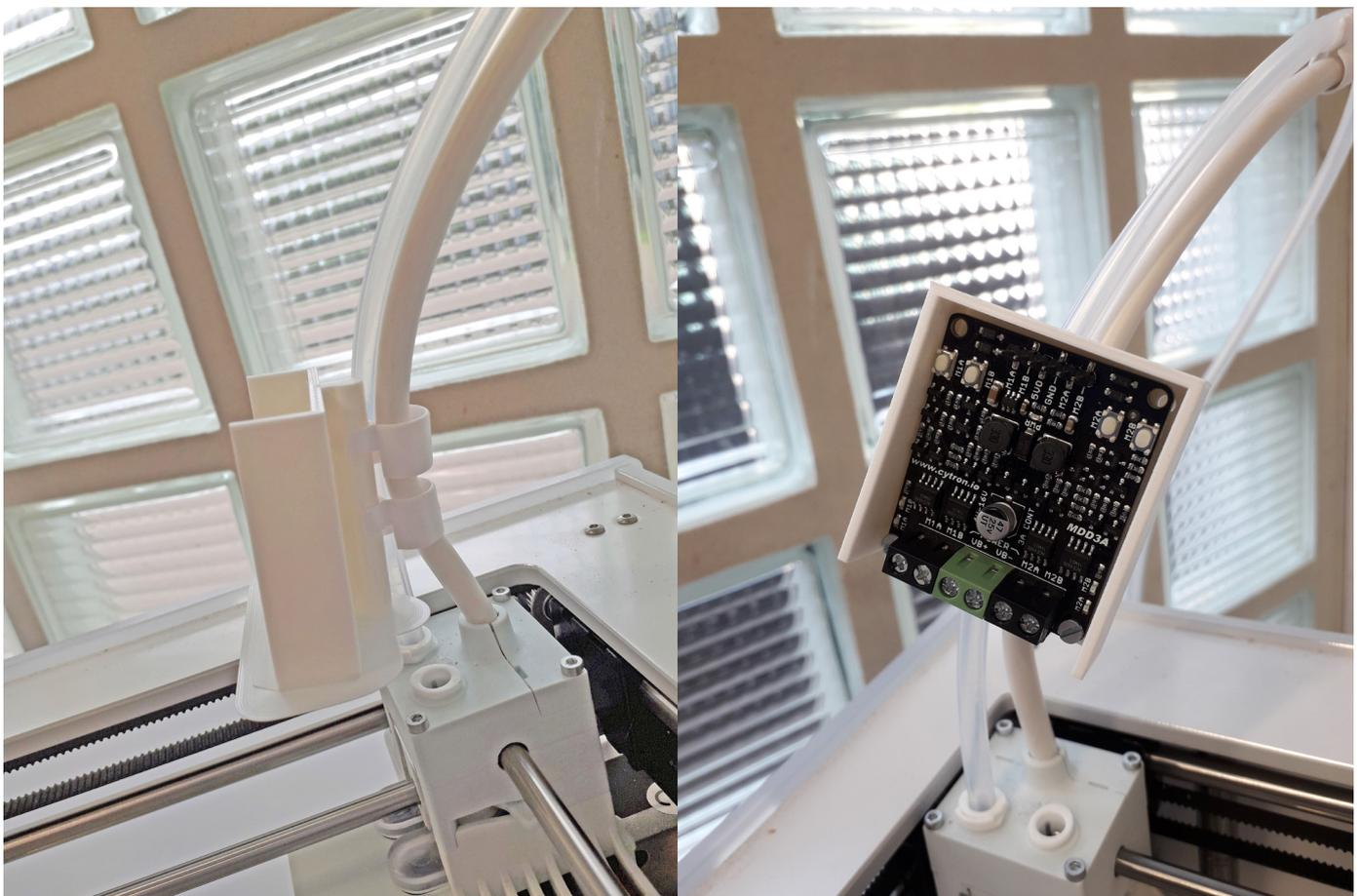
**Figure 3.42:** The connection piece of the H-bridge that can snap on the cable clips of the 3D printer
