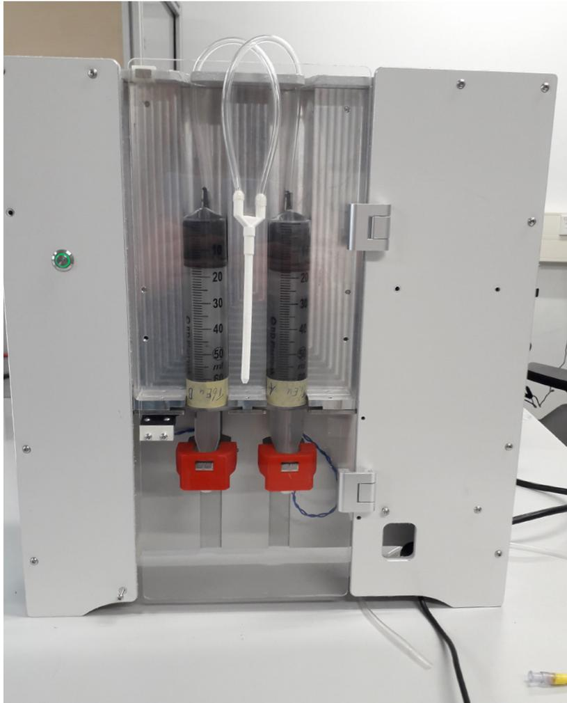
**Figure 3.28:** Dual syringe printer extruder. The two syringes both contain another ink component based on Ecoflex parts A and B. The tubes will guide the ink to the white static mixing nozzle (hanging between the syringes) where the two components are mixed.
