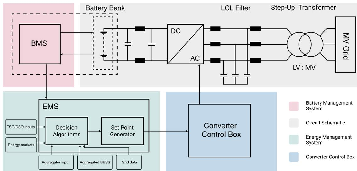
Figure 2.3: Circuit schematic of a grid-connected battery energy storage system with main components
