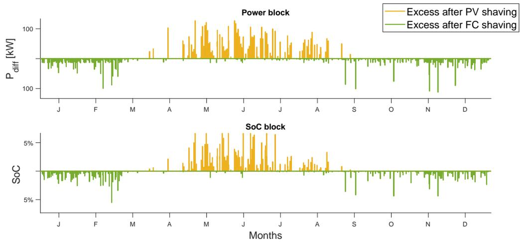
Figure 4.10: Example of Power block and SoC block profile obtained after have shaved 20% of the PV power and 40% of the FC station
