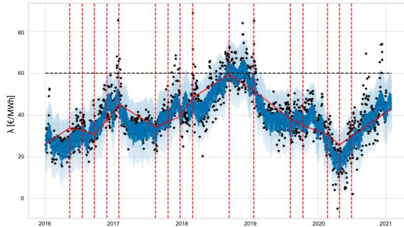
Figure 4.2: Daily electricity market data fitting from 2016 to 2021 (Netherlands). Segmented red line represents the trend. Vertical dashed red lines mark the trend change-points. Black dots mark the outliers
