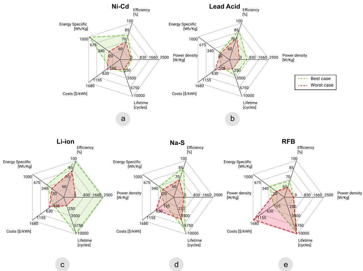
Figure 2.1: Comparison of power density, energy density, efficiency, costs and lifetime for the most popular battery storage technologies: (a) Nickel–Cadmium, (b) Lead Acid, (c) Lithium ion, (d) Sodium Sulfur and (e) Flow Battery - author's elaboration from [12] and [13]
