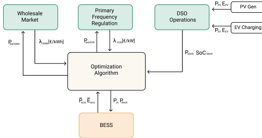
Figure 3.1: The model set up shows the virtual exchange of information among the different modules composing the optimization: Wholesale Market (DAM), Primary Frequency regulation (FCR), DSO operations and the BESS
