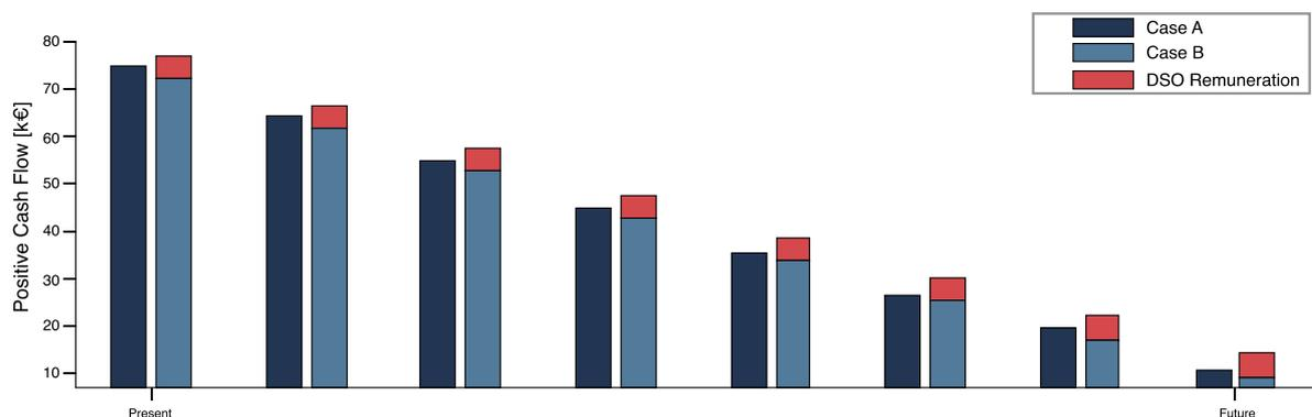
Figure 5.2: Projected cash flow of a 500kW/500kWh BESS operating in electricity markets and with DSO operation included. Case A indicates the cash flow coming only from market applications and Case B the cash flows with the DSO extra remuneration
