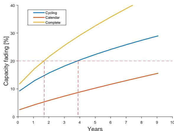
Figure 5.4: BESS lifetime projection. Complete degradation refers to the capacity fading due to cycling and due to aging (calendar). Capacity fading due to cycling occurs in 4 years with an overall lower than 2 years battery lifetime.
