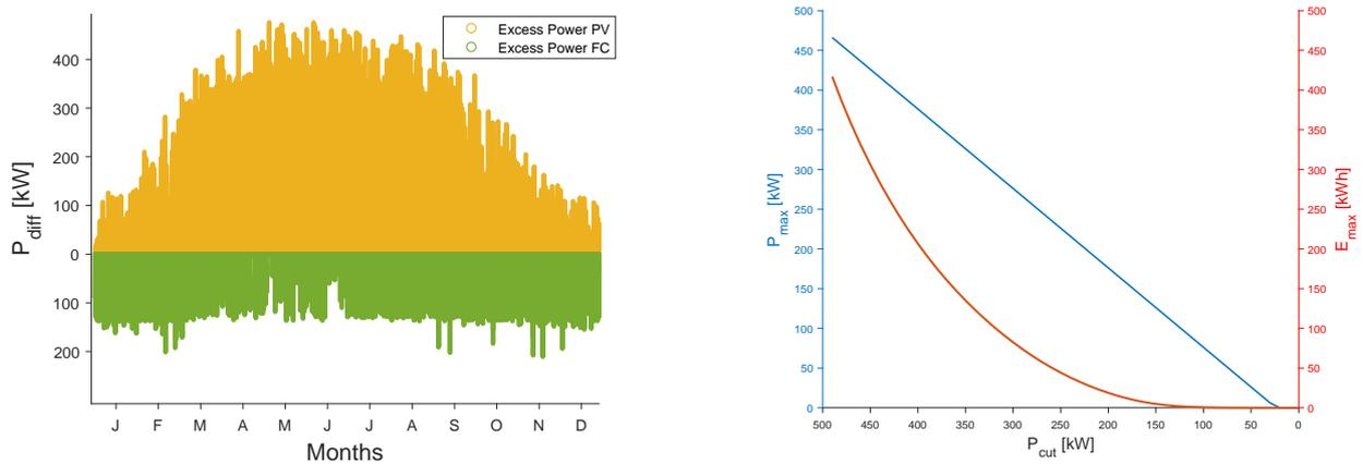
(a) PV-FC charging station power trend. The orange area above zero represents the excess power produced by the solar plant, while the green area is the extra power demand due to EV charging
