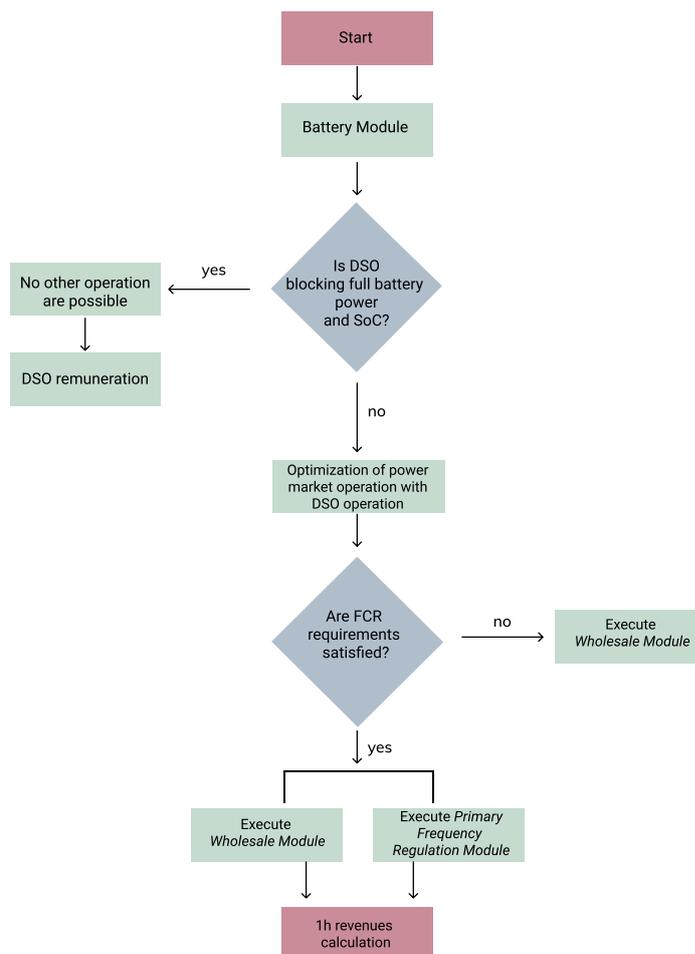
Figure 3.2: Flow chart of the algorithm. Every optimization timestep, the algorithm follows the logic displayed to maximize the revenues of the BESS. The DSO operation block is the first constraint. If full capacity is given to DSO, no other operations are possible. The execution of FCR is subjected to regulatory requirements. The execution of the wholesale module could help to fulfill them, maximizing the range of operations
