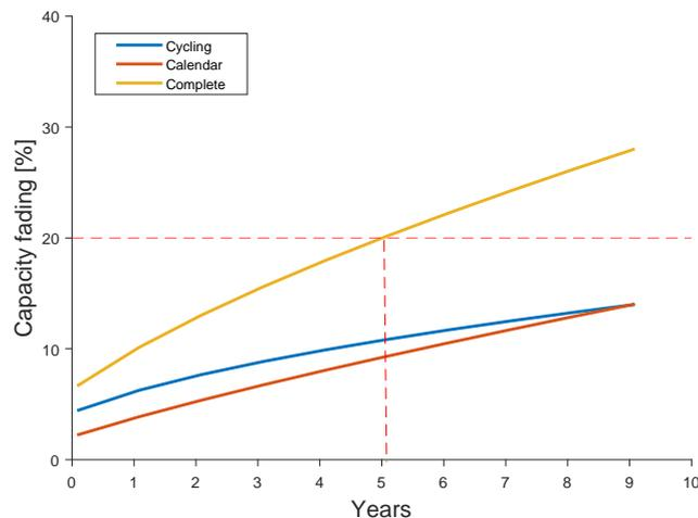
Figure 5.5: BESS lifetime projection with SoC limited to range 80%-20%. Complete degradation refers to the capacity fading due to cycling and due to aging (calendar). Overall improving in battery lifetime to more than 5 years.
