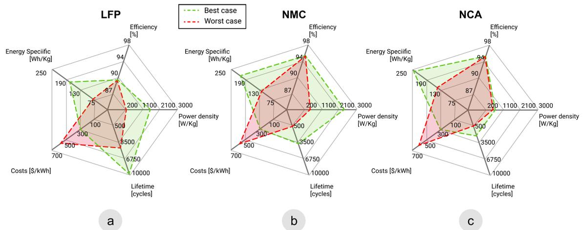
Figure 2.2: Comparison of power density, energy density, efficiency, costs and lifetime for the most popular Li-ion battery storage technologies for Grid applications: (a) Lithium Iron Phosphate, (b) Lithium Nickel Manganese Cobalt Oxide, (c) Lithium Nickel Cobalt Aluminum Oxide - author's elaboration from [12] and [13]
