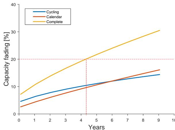
Figure 5.6: BESS lifetime projection using commercial Alphen BESS with SoC boundaries. Complete degradation refers to the capacity fading due to cycling and due to aging (calendar). Capacity fading due to cycling occurs after the BESS EoL. Overall lifetime between 4-5 years.
