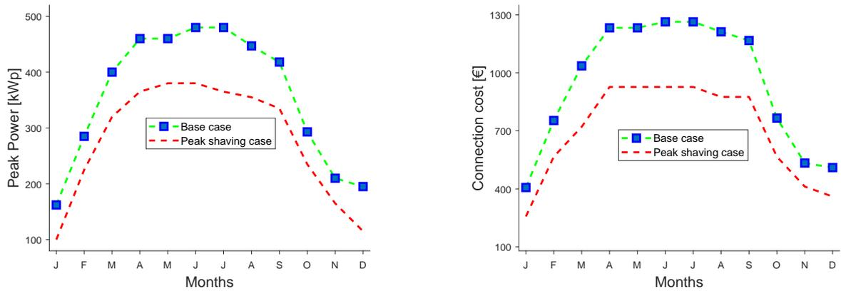
(a) Peak power grid exchange evaluation in normal condition (base case) and with BESS performing peak shaving
