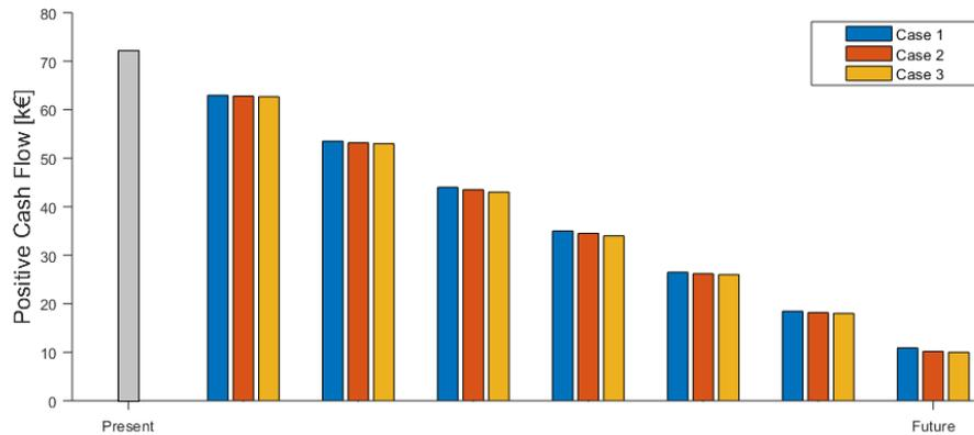
Figure 5.1: Projected cash flow of a 500kW/500kWh BESS operating in electricity markets. The revenues are based on the calculated 2020's one (in gray), scaled linearly to the future outcome. In blue the trend based on the forecasted dataset (Case 1), in red the trend based on the respective upper boundary (Case 2) of the dataset and in orange with the lower boundary (Case 3)
