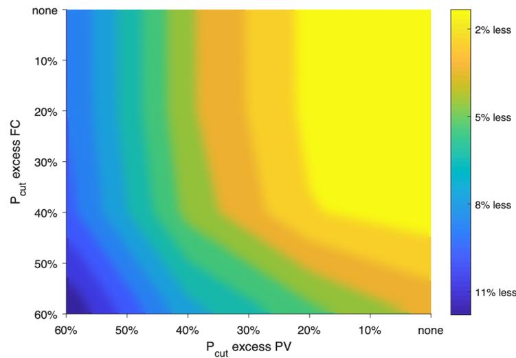
Figure 4.9: Revenues decrease depending on the power shaved from the PV-EV charging station
