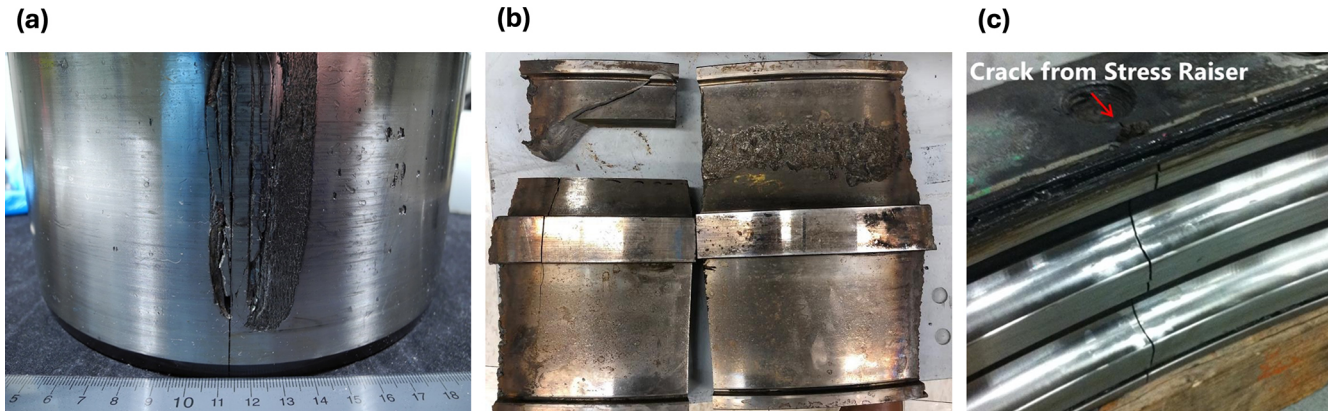
Figure 1. Examples of bearing cracks and damage in wind turbines. (a) Gearbox bearing WEC and spalling (Greco et al., 2022). (b) Main bearing WEC and spalling (Greco et al., 2022). (c) Pitch bearing ring crack (Shapiro, 2017).
