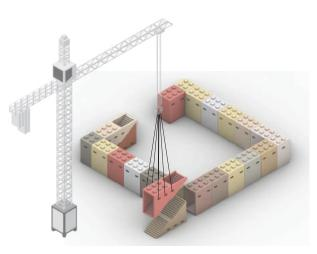
Place hollow stairs on the ground / Top part stacked on the bottom one.
