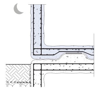
Thermal Comfort: Winter Active Insulation / Using the mass of the concrete to heat up the space
