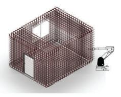
Prefabrication of the last horizontal reinforcement after door installation
