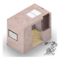
After the concrete is dried, the element is flipped 90 degrees in order to apply concrete on the roof
