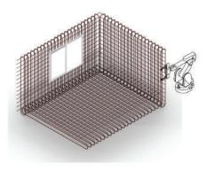
Assemblage of the different sides of the concrete element
