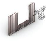
Prefabrication of vertical reinforcement
