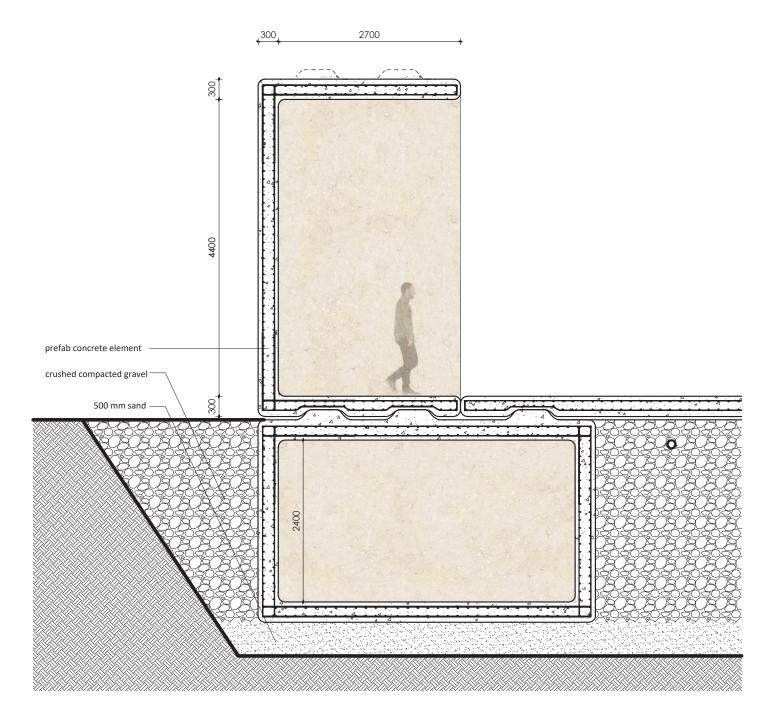
detail: Interlocking Structure scale 1:20
