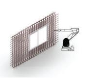
Prefabrication of horizontal reinforcement via Novel robotic wire application
