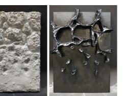
Composition: Gap-graded aggregates Thin layer of cement paste Void
