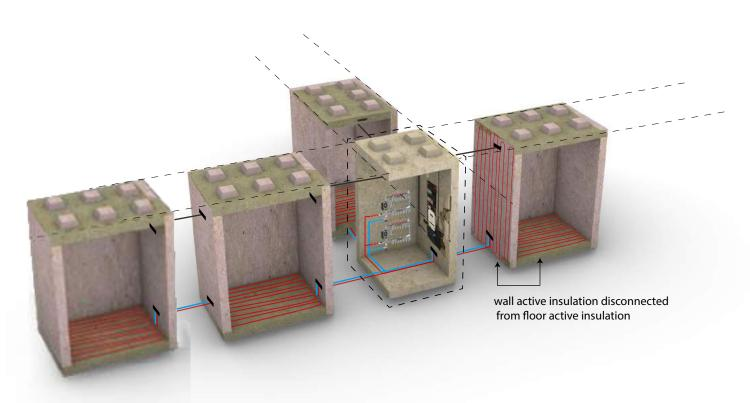
One concrete element can be used as a technical room. Water pipes and electricity instllations are connected to the technical room via openings on the concrete Openings can be used for servises or ventilation
