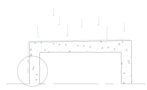
Roof has an inclination of 1 degree in order for the rain water to leave the roof of the concrete element and fall on the ground
