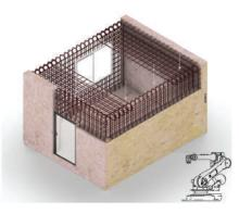
Concrete spraying using the robotic arm. The robot first applies the concrete on the inside of the element and customises each side according to a specific colour
