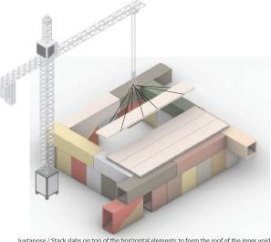
Juxtapose / Stack slabs on top of the horizontal elements to form the roof of the inner void
