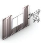
Existing window re-used and places within the fabricated opening
