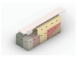
5. Stack orthogonal slab on top of the horizontal element (inhabitable beam)
