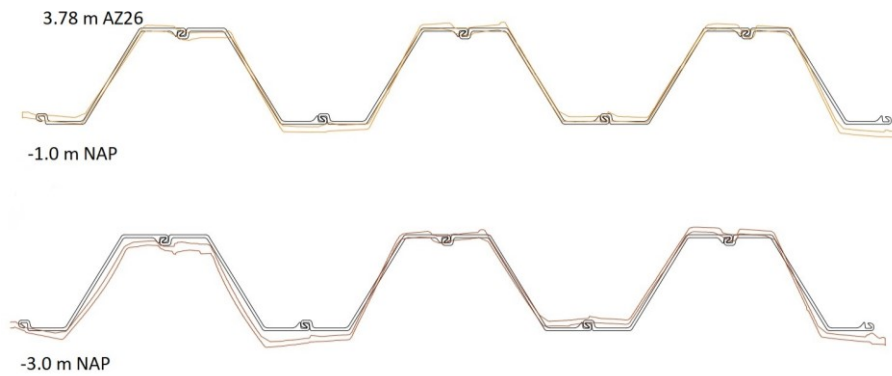
Figure 4.28 GU8N: Deflections and curvature of middle (blue) and side (orange) sheet pile
