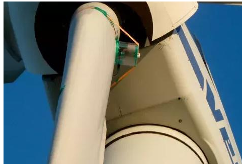
Figure 1.10: A vibration measurement system for blade health monitoring [39].
