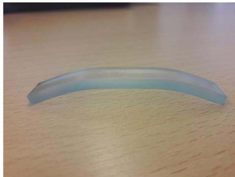
Figure 4.4: Photograph of the a highly deformed epoxy resin specimen after a stress relaxation test.
