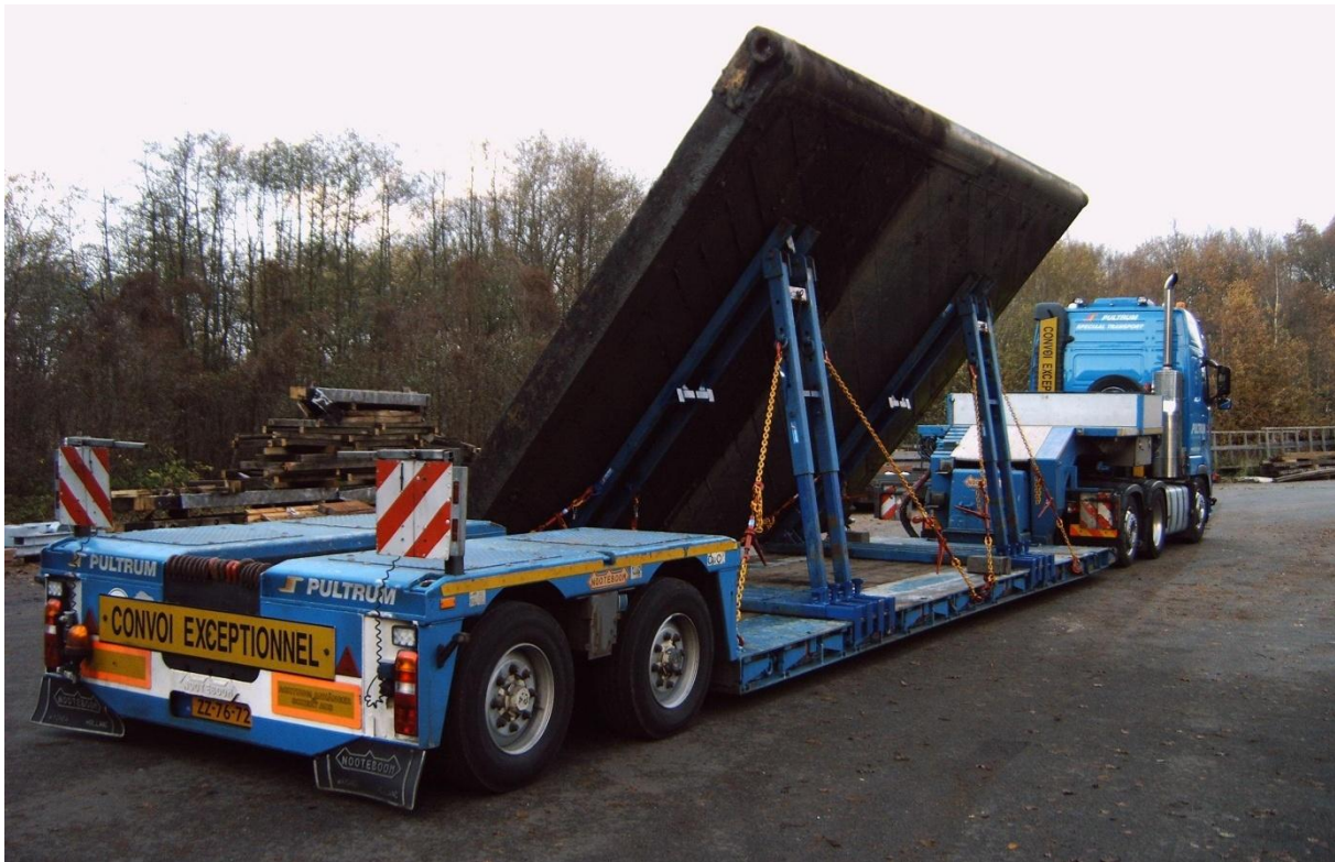
Figure 160 Flatbed trailer with a sluice door at an angle [Pultrum 2012]
