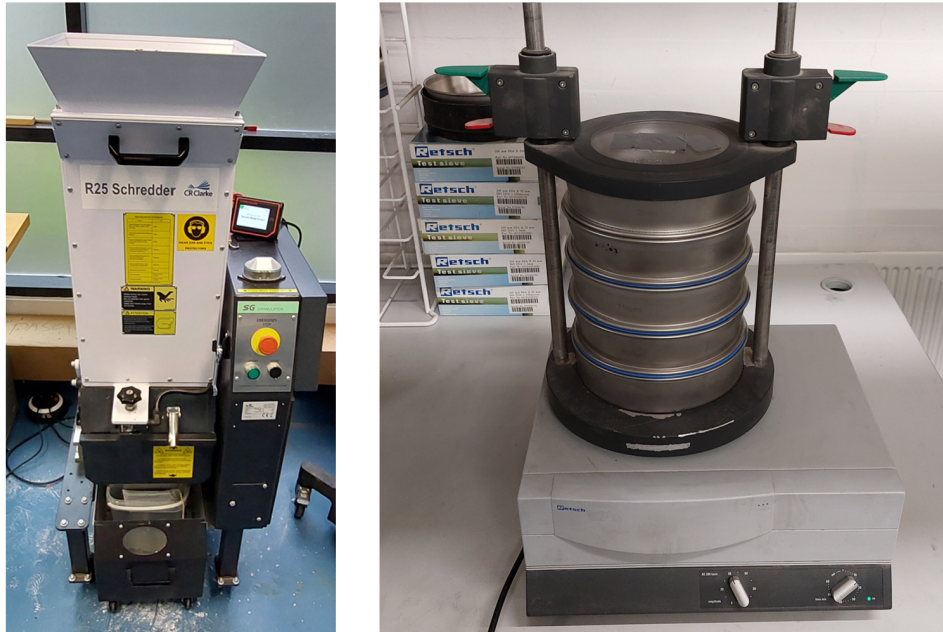
Figure 19: R25 Granulator (left) and Retsch AS 200 Basic Sieving Machine (right)
