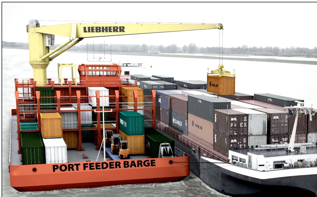
Fig. 13: The Port Feeder Barge is serving an inland barge midstream (computer rendering)
