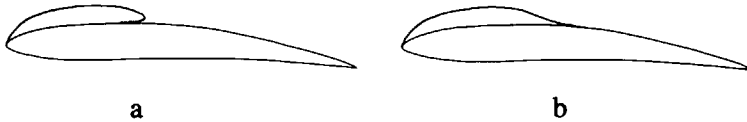
Figure 2.2: Schematics of the possible topology for reattachment for 2-dimensional steady cavity flow. a) tangential with body surface but travels upstream; b) tangential with body surface but travels downstream.
