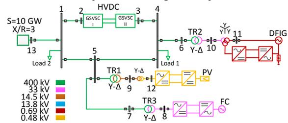
Fig. 2. Test network for studying protection performance.
