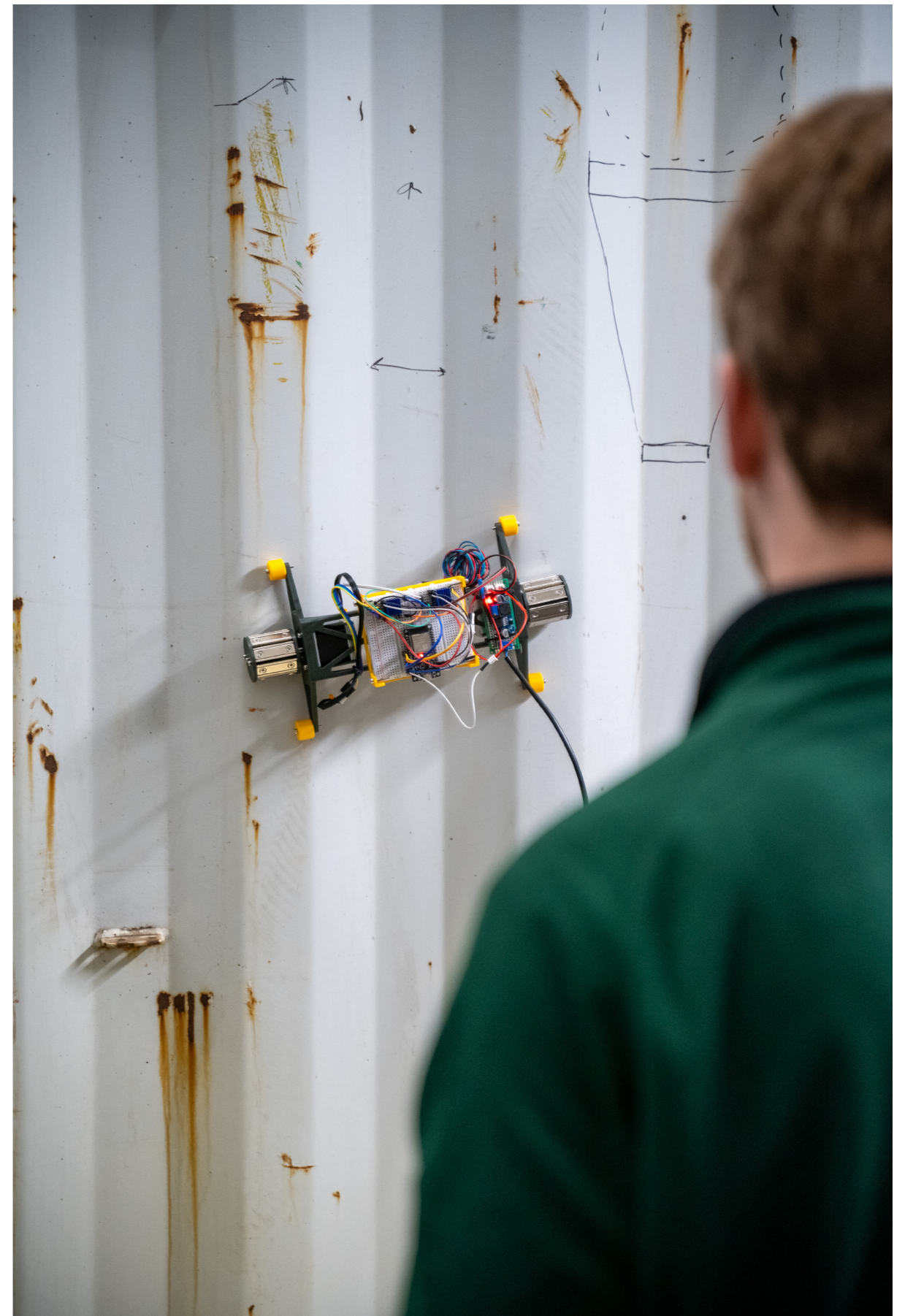
Figure 38 – Driving over container wall
