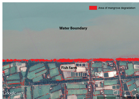
Figure 1. Mangrove degradation along a straight part of Dinh An estuary, An Thanh province, Vietnam. The red area illustrates the area loss of mangrove from 2006 to 2014. Fish farms constructed close to the water boundary push the mangrove into a narrow fringe zone. This area is suffering from erosion with a rate of about 2.5 \text{ m yr}^{-1} [2].
