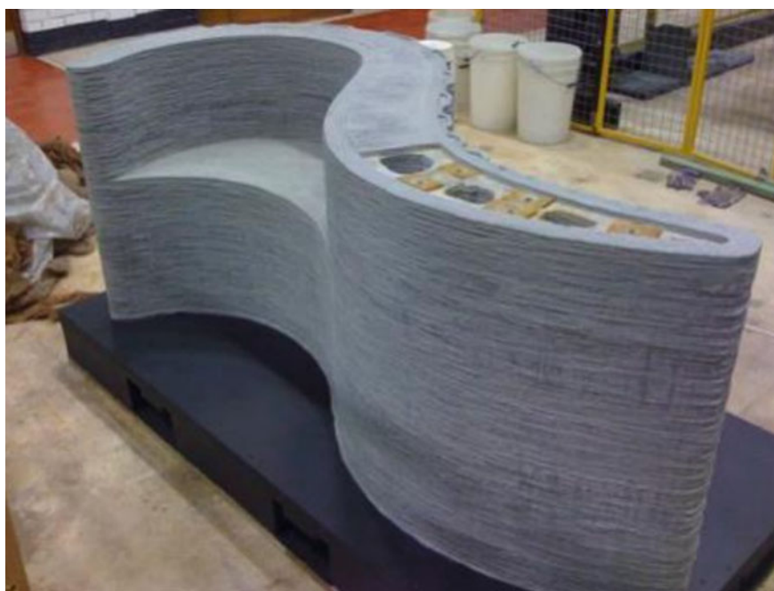
Fig. 6.9 Digital manufacturing of a free-shaped wall-like concrete bench (Buswell et al. 2018)
