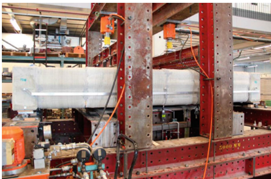
Fig. 6.13 Scale model in test 4-point bending test set-up (Theo et al. 2018)
